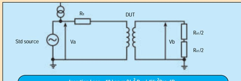
$$\text{Insertion Loss} = 10 \text{ Log }_{10} (V_a^2 \text{ Ret} / 4V_b^2 \text{ Rit}) \text{ dB}$$
