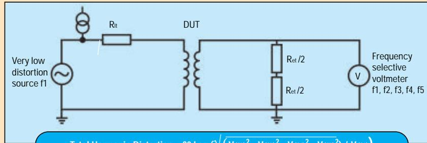
$$\text{Total Harmonic Distortion} = 20 \text{ Log } \left( \sqrt{V_{(f2)}^2 + V_{(f3)}^2 + V_{(f4)}^2 + V_{(f5)}^2} / V_{(f1)} \right)$$
