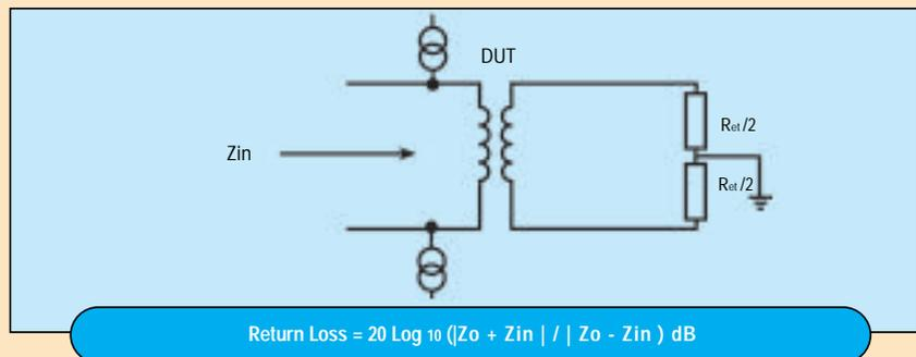
$$\text{Return Loss} = 20 \text{ Log }_{10} (|Z_o + Z_{in}| / |Z_o - Z_{in}|) \text{ dB}$$
