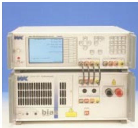
*3265A seen here being used with the PMA3260A Precision Magnetics Analyser*
