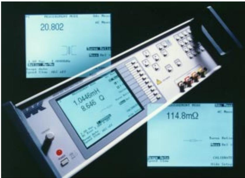
**The IA3255 Inductance Analyzer is designed to appeal to users who design and manufacture inductors and transformers and are looking for high performance and value for money. Lightweight and portable, the IA3255 includes many features - such as an extensive range of measurement functions, fast testing speeds, wide frequency range and full remote control - typically associated with more expensive units.**
