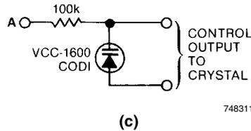
**FIGURE 8.** Stable quartz-crystal oscillators can operate with a single active device (a). You can achieve maximum frequency stability by mounting the oscillator in an oven and using a temperature-controlling circuit (b). A varactor network (c) can also accomplish crystal fine tuning. Here, the varactor replaces the oven and retunes the crystal by changing its load capacitances.
