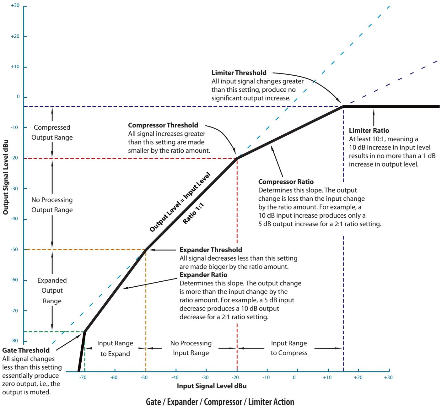
dBu and a musical peak suddenly comes along and causes the input to jump by 10 dB to +26 dB, the output will only increase by 1 dB to +17 dBu — basically remaining level. Limiters find use in preventing equipment and recording media overloads. A limiter is the extreme case of compression.
