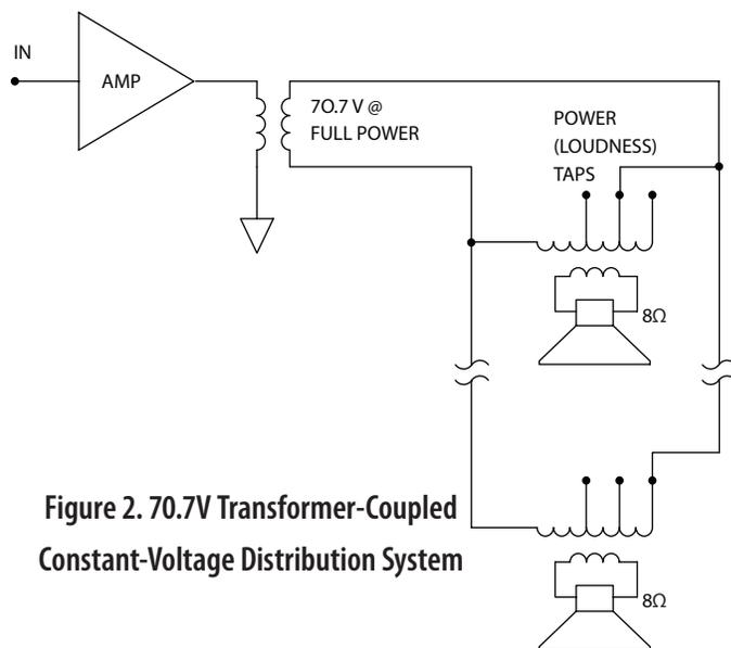
Figure 2. 70.7V Transformer-Coupled Constant-Voltage Distribution System
