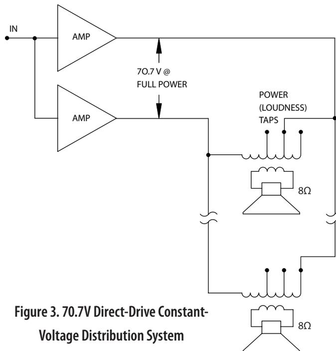
Figure 3. 70.7V Direct-Drive Constant-Voltage Distribution System
