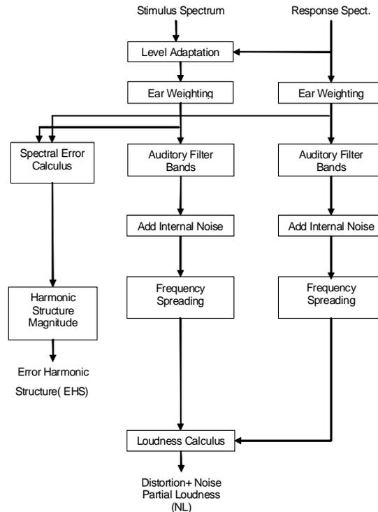
Figure 11: Overall flowchart of our PEAQ algorithm
