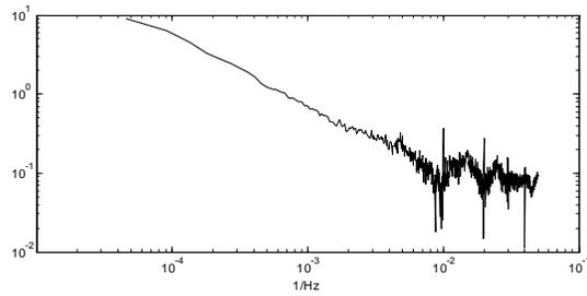
**Figure 19: Power Cepstrum of Borderline loudspeaker (EHS = 0.37)**
