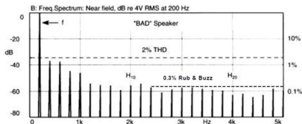
**Figure 3: Waveform spectrum of the output of a “bad” loudspeaker exhibiting high Rub & Buzz distortion. Note the high level of high-order harmonics. THD = 2 %, Rub & Buzz distortion = 0.3 %. This driver exhibits a buzz due to a rubbing voice coil as a result of a bent frame.**
