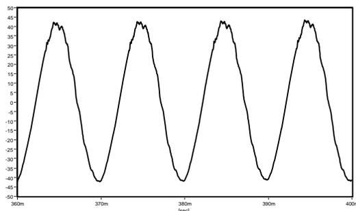
**Figure 1: Acoustic output waveform of a loudspeaker exhibiting high levels of Rub & Buzz distortion when driven by a sine wave. Note the waveform anomalies on the top and bottom of each cycle of the sine wave.**
