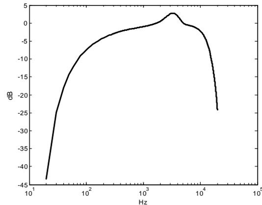
**Figure 5: Outer and Middle Ear Frequency Characteristic**
