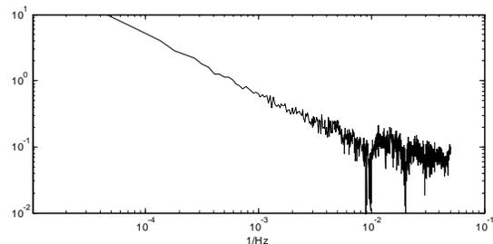
**Figure 18: Power Cepstrum of Good loudspeaker (EHS = 0.13)**
