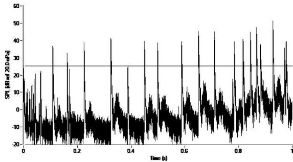
Figure 8: Speaker with Loose-particles. #LP: 48
