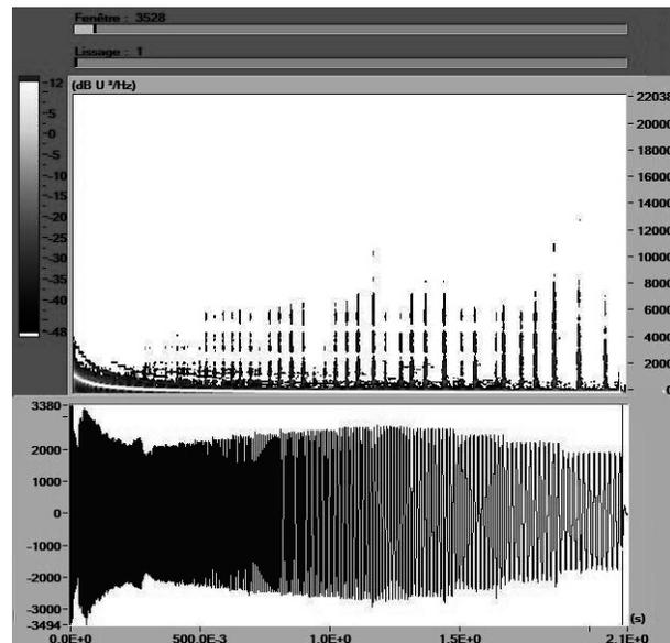
Figure 3: Loose Particles
