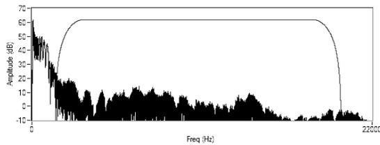
Figure 14: Spectrum of LP Speaker response + filter window
