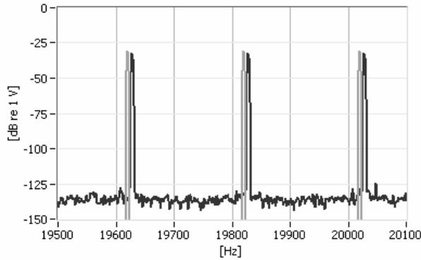
Figure 4 Response Spectrum (dark) vs. Stimulus Spectrum (light)
