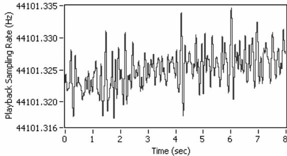
Figure 5 Jitter - Instantaneous Sampling Rate vs. Time
