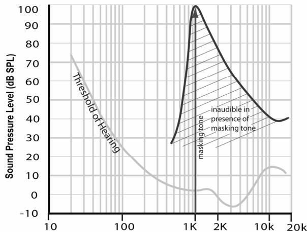
Figure 2 Masking curve used to eliminate 'unheard' sounds
