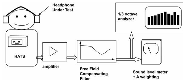
Figure 15 Test equipment requirements according to BS EN 50332
