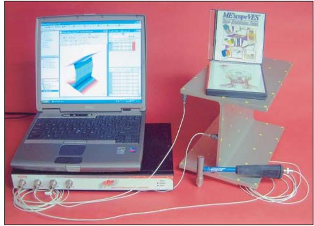
*ME'scopeVES* uses Vibration Research 8500 shaker-controller to acquire impact data.
