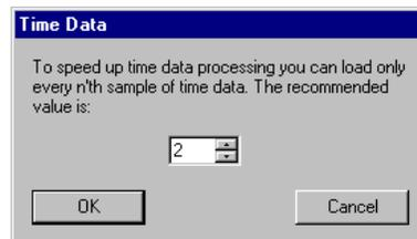
Figure 8.3: Dialog for reducing the time data step size
