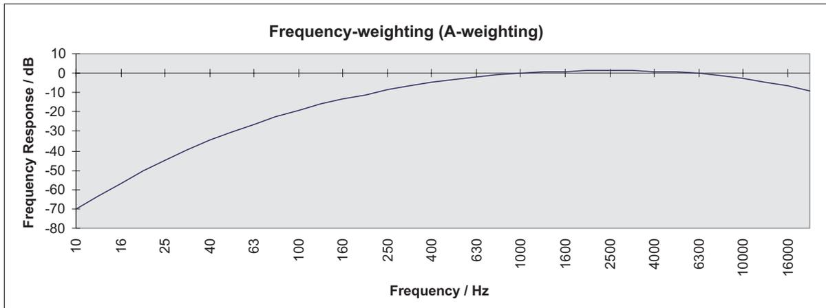
Figure 7.9: Frequency-weighting curve for the display type Magnitude[dB(A)]
