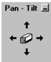
You control the motorized pan-tilt stage with the icons **Pan-Tilt**. If you can not see the icons in the scanning head control, then first of all activate the pan-tilt stage for the software. See [chapter 2](#) on this.
