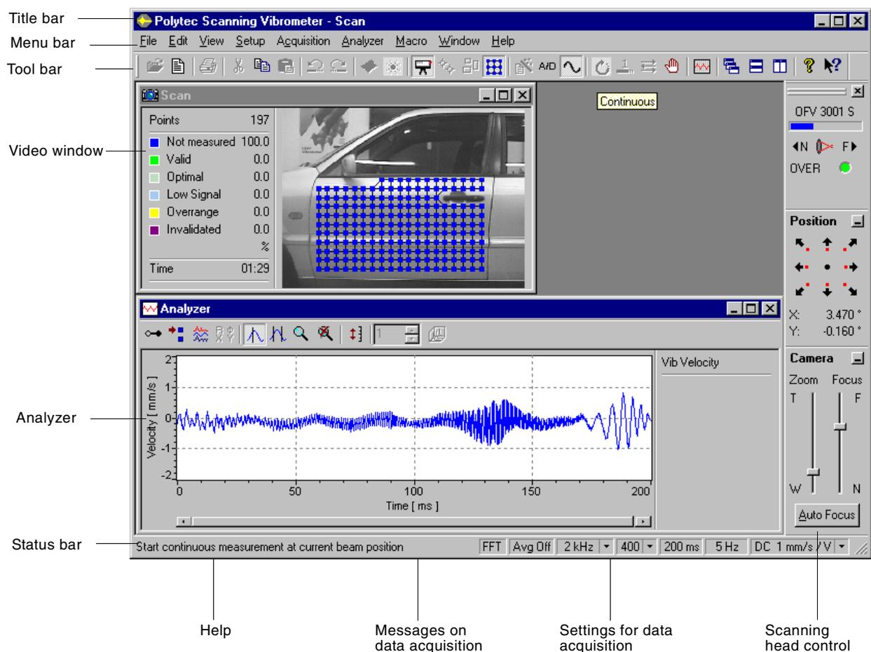
Figure 1.2: Example of the application window in acquisition mode
