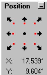
You move the laser beam with the icons **Position**. To do so, click the icon for the direction required. If you click , then the laser beam is positioned so that it is emitted at a right angle to the front panel of the scanning head (position 0; 0). Below the icons you can see the current position of the laser beam.
