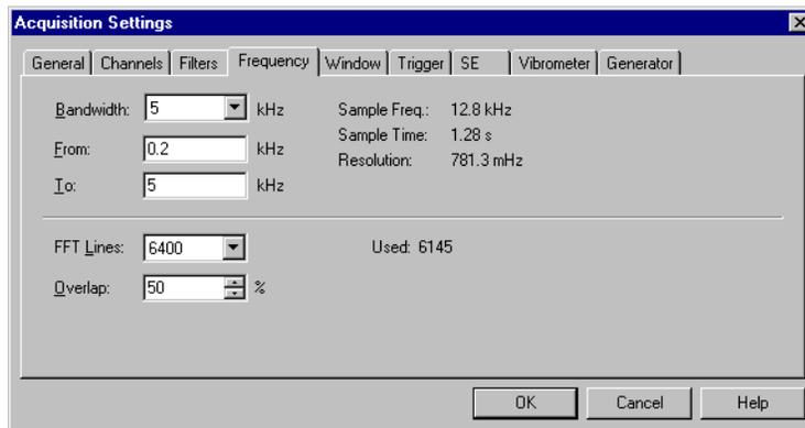
Figure 6.5: Page Frequency in the measurement mode FFT
