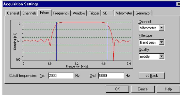
Figure 6.4: Page Filters, part 2 to set the parameters
