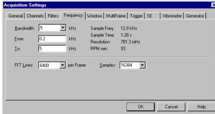
Figure 6.15: Page Frequency in the measurement mode MultiFrame
