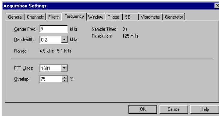
Figure 6.11: Page Frequency in the measurement mode Zoom-FFT
