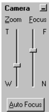
You zoom the video camera with the slider **Zoom**. Using the mouse you can roughly set the slider. If the slider is active, you can fine-tune it with the arrow keys  $\uparrow$  and  $\downarrow$ . (To activate the slider, click it.)
