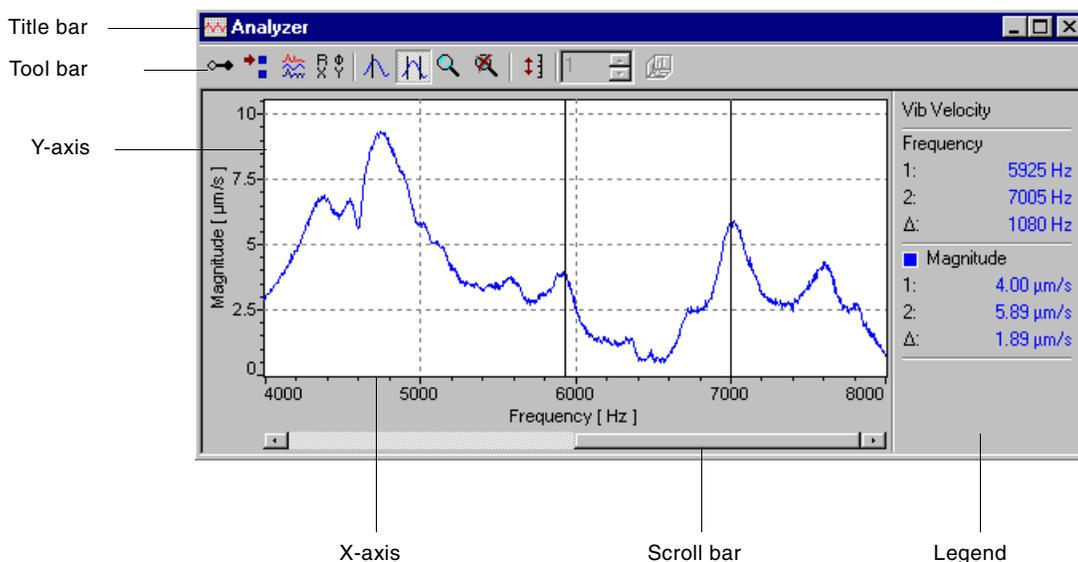
Figure 1.4: Example of an analyzer
