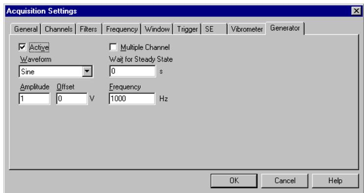
Figure 6.10: Page Generator with user defined waveform
