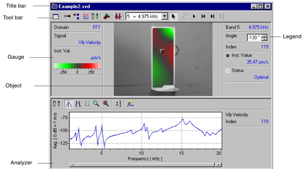
Figure 1.5: Example of a presentation window in the Single Scan Point view
