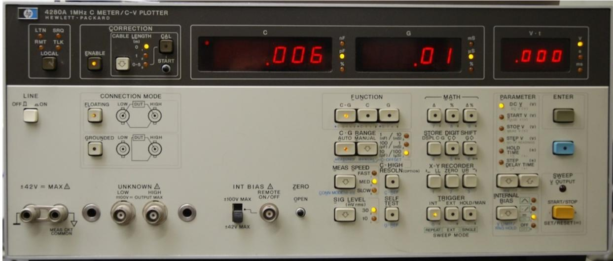
Figure 2. Front panel of the Hewlett-Packard 4280 capacitance-voltage meter.
