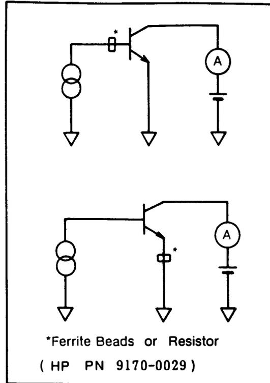
Figure 3. Preventing Transistor Oscillation
