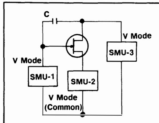
Figure 1. Test Configuration
