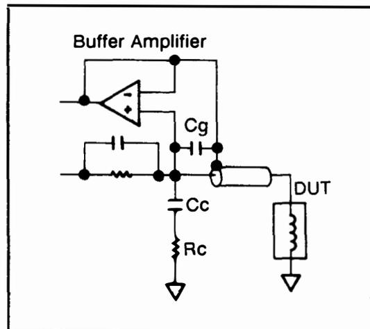
Figure 2. SMU Output Circuit
