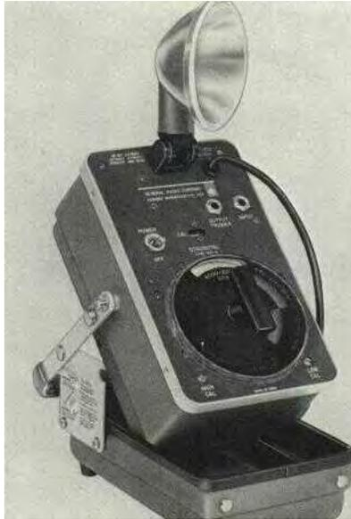
1531-A Strobotac® Electronic Stroboscope
