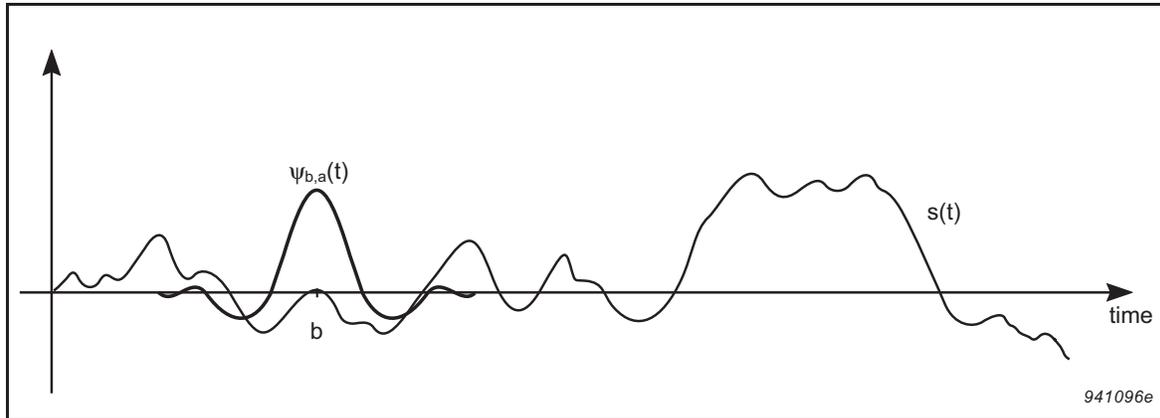
*Fig. 2. The Wavelet Transform (WT). The Wavelet,  $\psi$ , extracts time-scaled information from the signal,  $s(t)$ , around the time  $b$  by means of inner products between the signal and scaled (parameter  $a$ ) versions of the wavelet*
