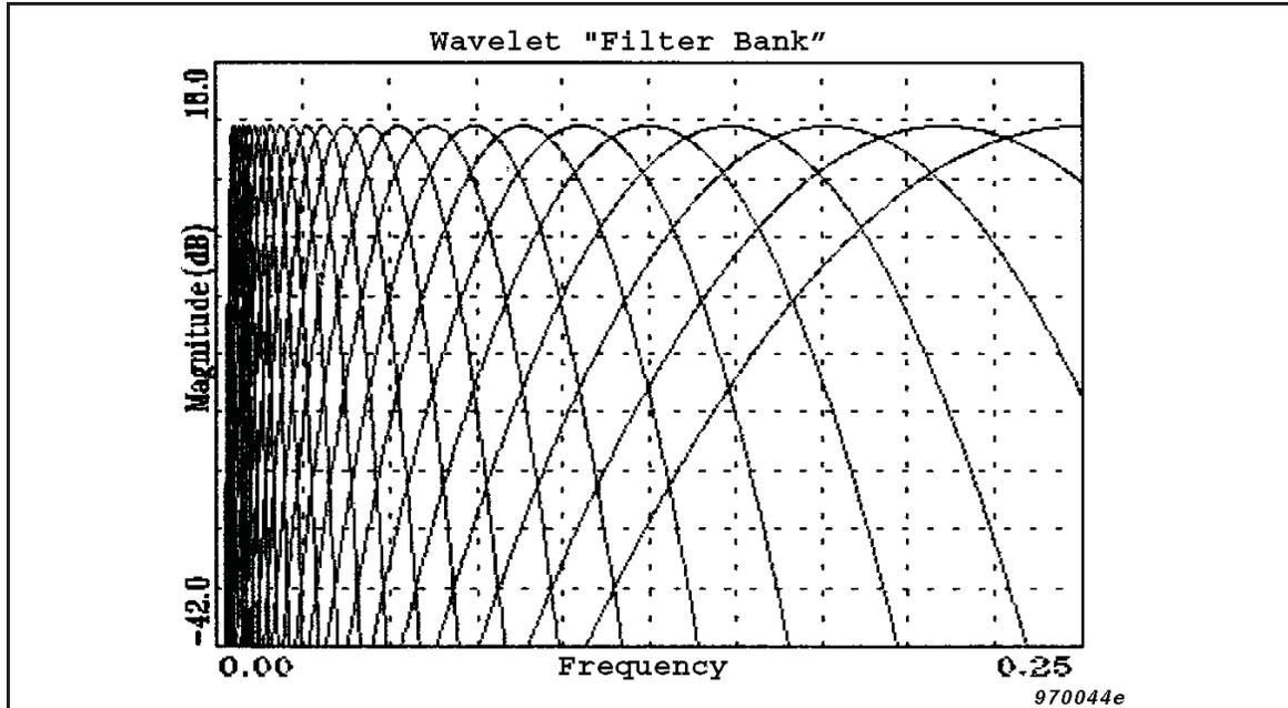
Fig. 15. 1/3-octave Wavelet “filter bank”, linear frequency
