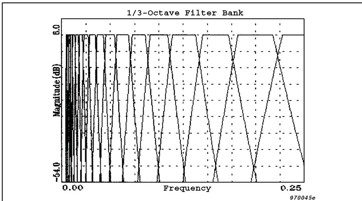
Fig. 14. Standardized 1/3-octave filter bank, linear frequency
