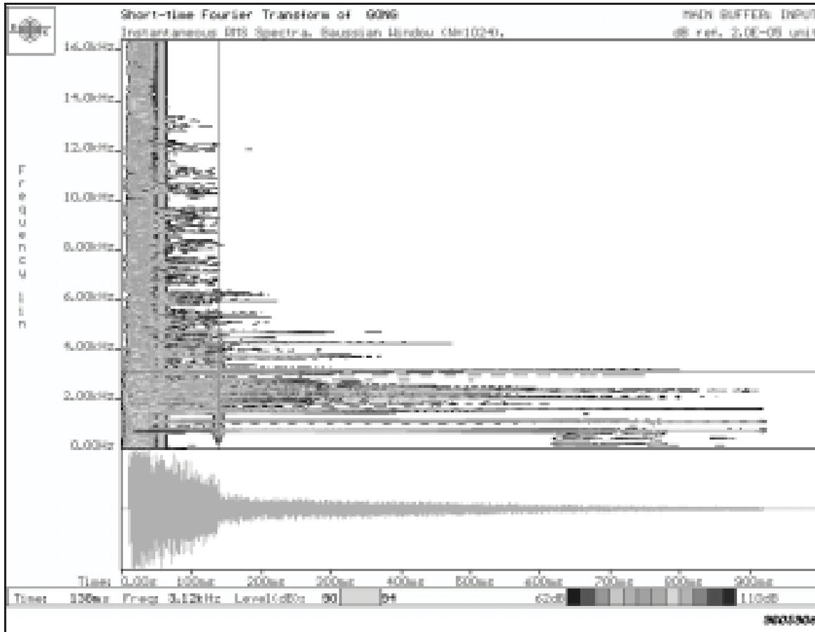
Fig. 3. A Short-time Fourier Transform of a free vibration decay measurement of a gong.  $2\Delta f = 50 \text{ Hz}$ ,  $2\Delta t = 6.3 \text{ ms}$ . A slice cursor can be used to extract the decay curve of the resonances for damping calculations
