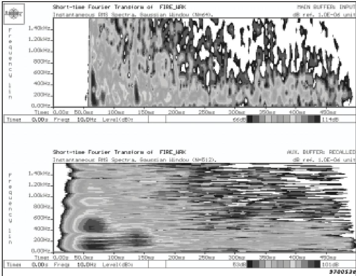
Fig. 13. Upper. An explosion analyzed with a small transform (STFT,  $N=64$ ) in order to obtain good time resolution,  $2\Delta t = 3.16$  ms
