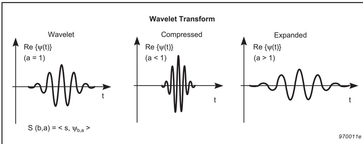
*Fig. 8. The basic wavelet contains a fixed number ( chosen by the user) of oscillations. The wavelet is then compressed/expanded in order to extract higher and lower frequency contents respectively*
