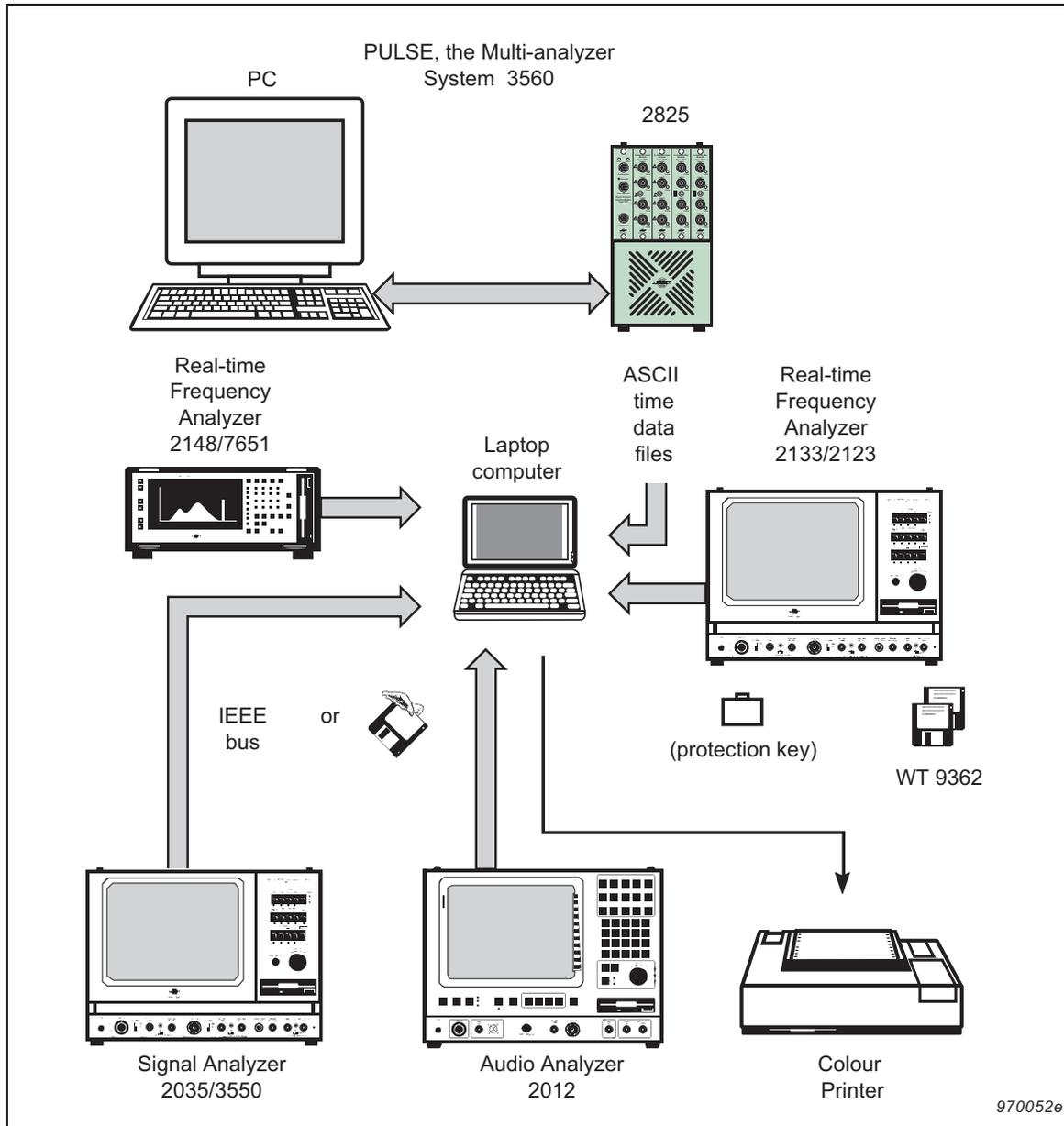
*Fig. 21. Data import to the “Non-stationary Signal Analysis Software” is possible from most Brüel & Kjær Analyzers. Export of data can be done using file-formatting programs such as HiJaak Pro which runs under MS-Windows*
