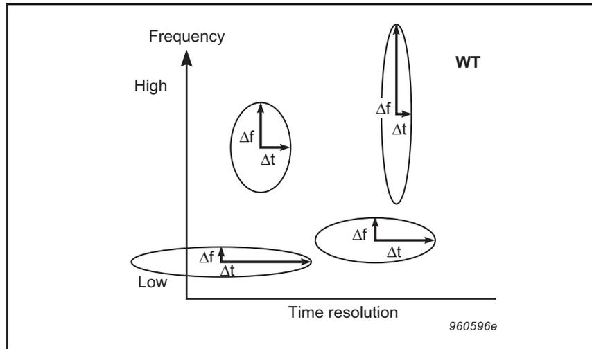
Fig. 10. Heisenberg's ellipses for WT. Y-axis is both a frequency and a frequency resolution axis
