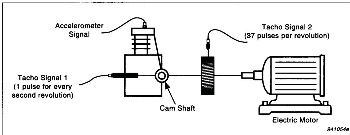
*Fig. 21 Test set-up. Tacho signal 1 used to trigger time records and for order tracking
