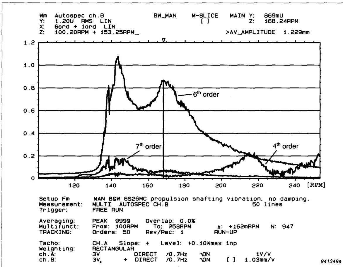
Fig. 15 Measurement set-up and analysis of undamped vibrations
