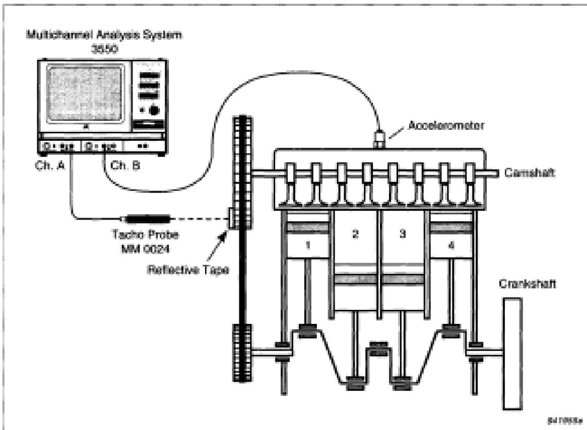
Fig. 17 Engine outline and measurement set-up
