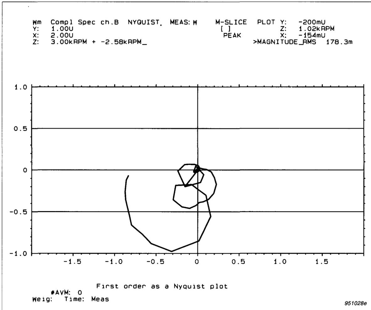
Fig. 11 Nyquist plot of the fundamental of generator vibration during coast down
