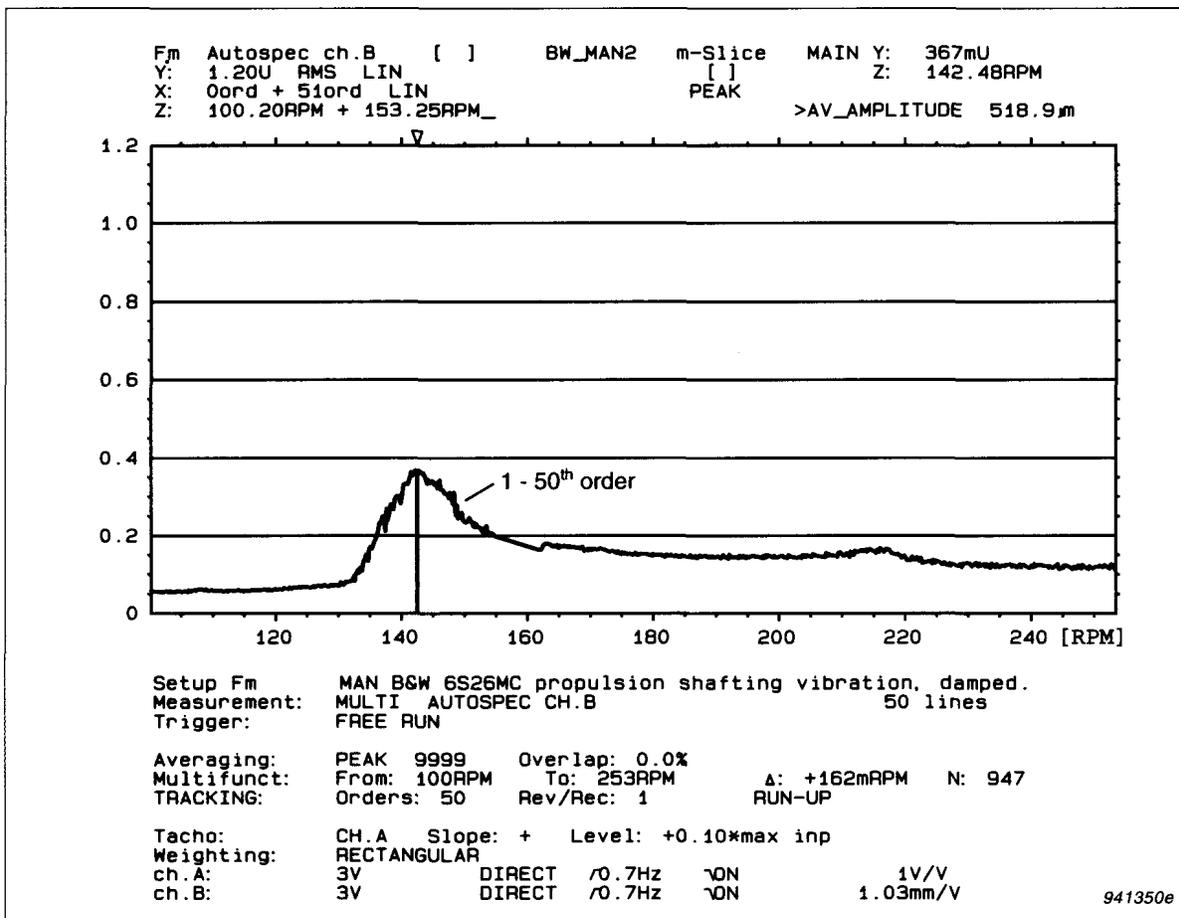
Fig. 16 Analysis of damped vibrations
