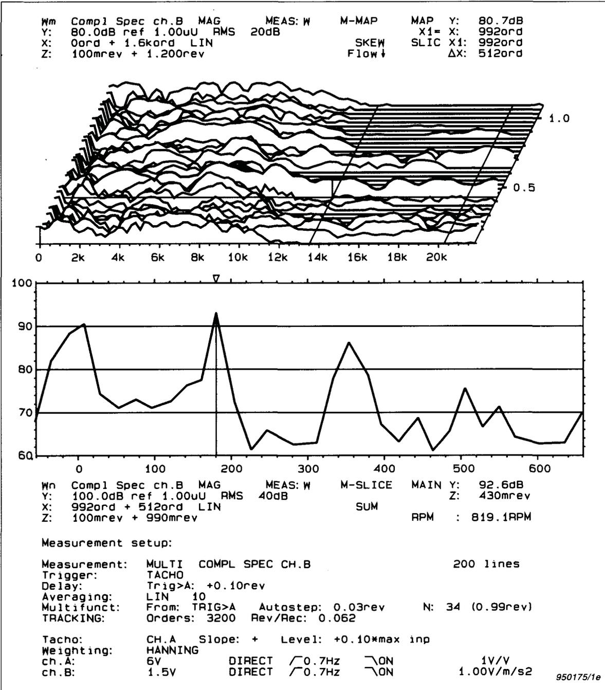
Fig. 20 Order Spectrum MAP and  $\Delta$ -SLICE of the gated, tracked vibration spectrum
