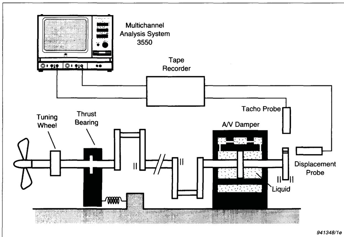
Fig. 14 Propulsion shafting model and instrumentation set-up
