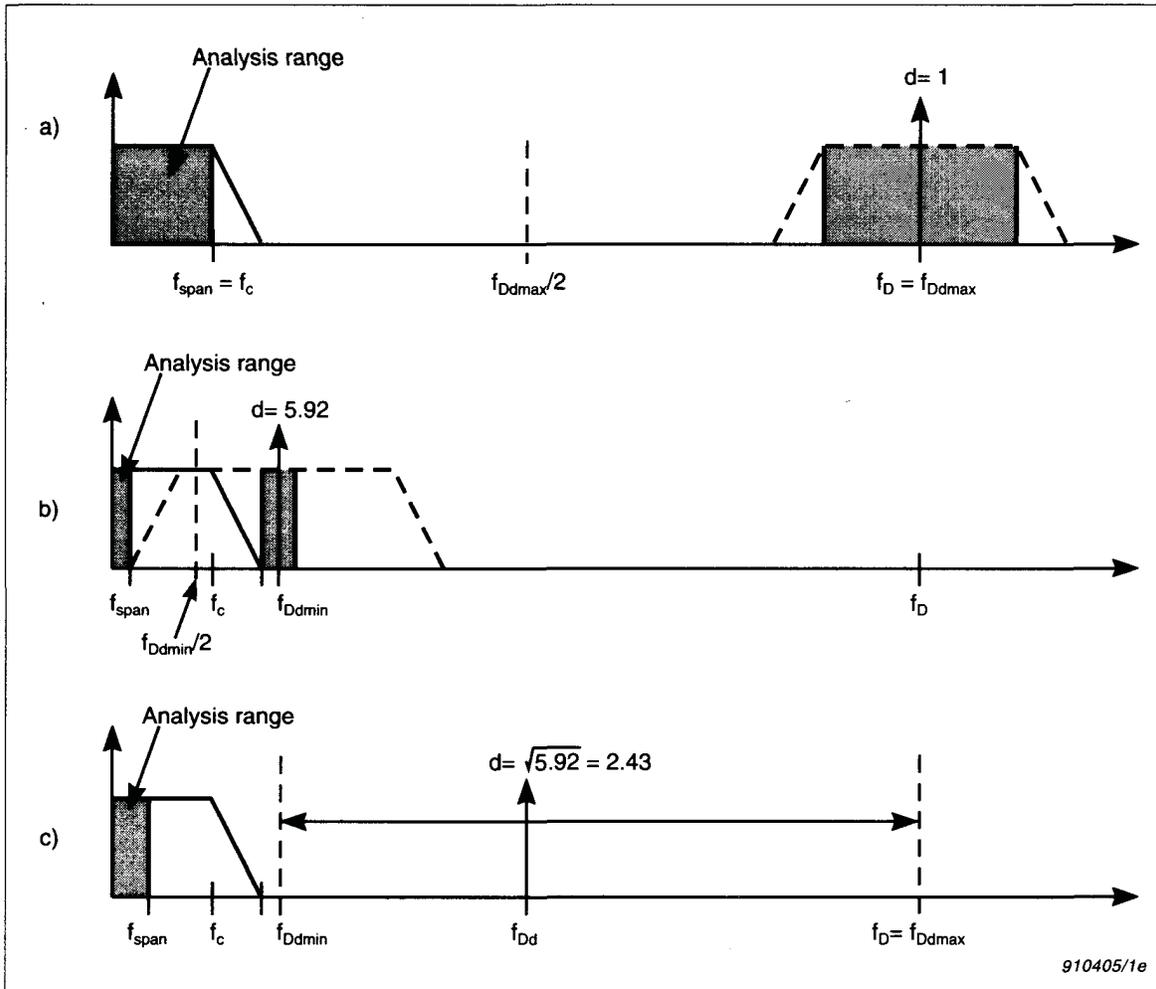
Fig. 5. Sampling frequency after decimation  $D$  in zoom processor  $f_D$ , sampling frequency after decimation  $d$  (interpolation and resampling)  $f_{Dd}$ , cutoff frequency of antialiasing filter  $f_c$  and analyzed frequency span  $f_{span}$  in the order analysis
