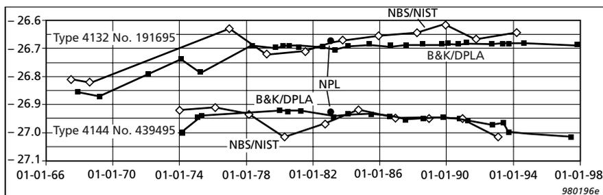
Fig. 11. Calibration results (250 Hz) obtained by NIST and by B&K. During the time of Type 4143 and its successor (since 1977) the spread of the B&K results has been small. During the same time the overall average of the deviations between the two laboratories has been very good. Between 1967 and 1977 the Type 4132 microphone has seemingly changed sensitivity
