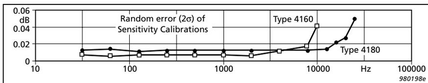
Fig. 14. Random calibration errors ( $2\sigma$  deviations from linear regression lines) as a function of frequency. The errors are calculated for the above-mentioned one inch and half inch microphones
