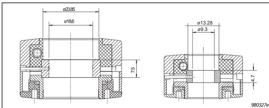
*Fig. 8. Plane-wave couplers for IEC 61094-1 LS1 (1") and LS2 (1/2") microphones. To ensure the highest possible stability the critical part of the couplers are made of single crystal sapphire. Type 9699 contains two couplers for each size of microphone. This makes it possible to estimate microphone volumes*
