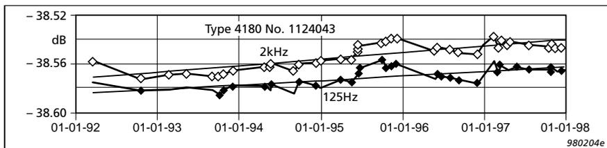
Fig. 13. Reciprocity calibration results (125 Hz and 2 kHz) obtained with a half inch microphone Type 4180. The deviations ( $2\sigma$ ) from the linear regression lines are  $< 0.012$  dB over a period of 6 years
