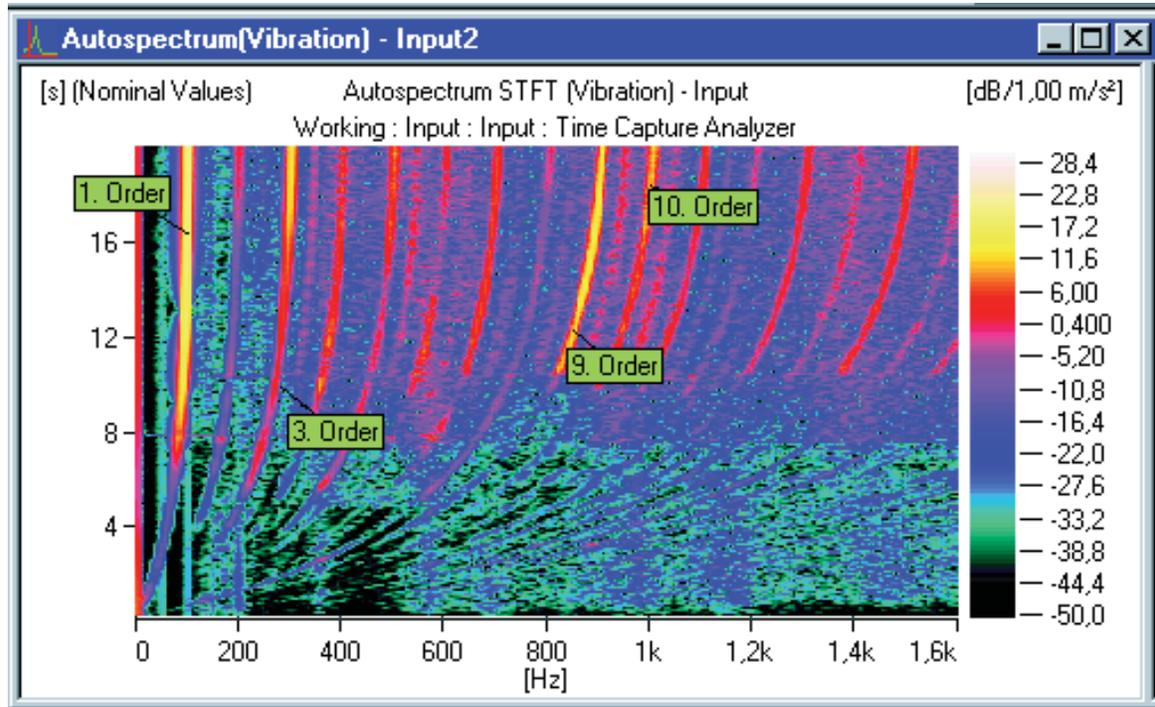
Fig. 11. An STFT of the vibration signal
