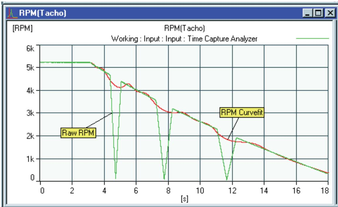
Fig. 8. Raw data and spline fit
