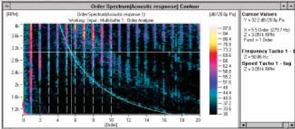
Fig. 5. Contour plot of real-time order tracking spectra (resampling technique) of the acoustic response
