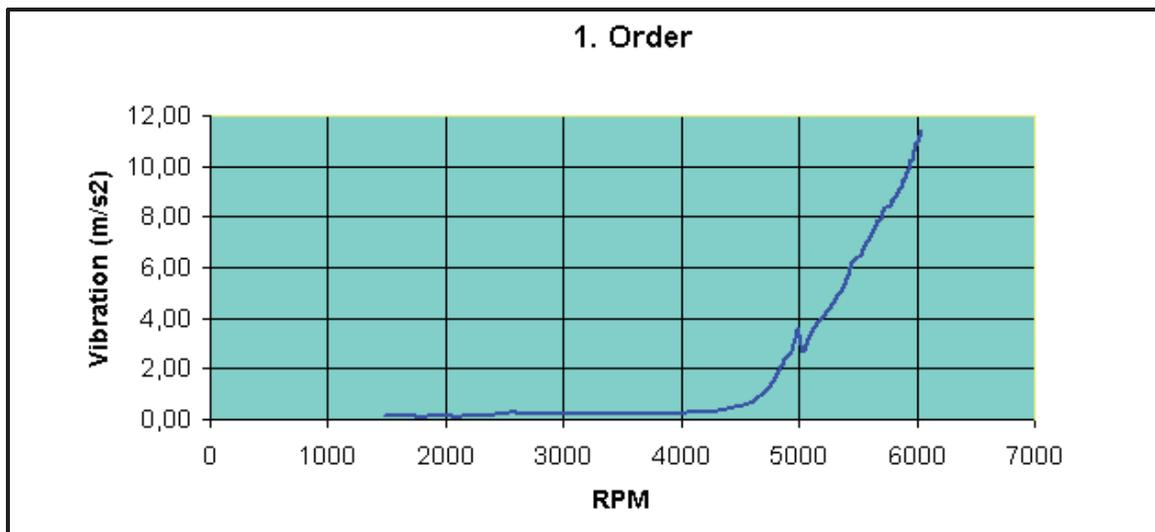
Fig. 18. Magnitude of the first order as a function of RPM, extracted using a two-pole Vold-Kalman filter with 10% bandwidth and plotted via MS Excel spreadsheet
