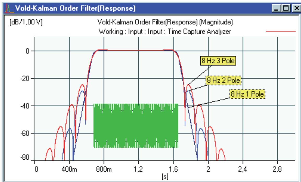
Fig. 21. Comparison of the magnitude of the time responses for one-, two- and three-pole Vold-Kalman filters with a bandwidth of 8 Hz. The applied signal, a tone burst of 1 s duration, is shown as well
