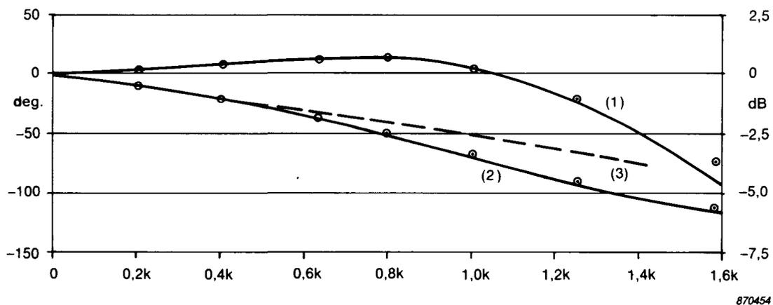
Fig. 3 Magnitude difference (1) and phase difference (2) between the pressure of the calibrator cavities, (b)-(a) were measured (curves) and calculated (points). The dotted line (3) shows the free-field phase lag for points 50 mm apart at 20° C
