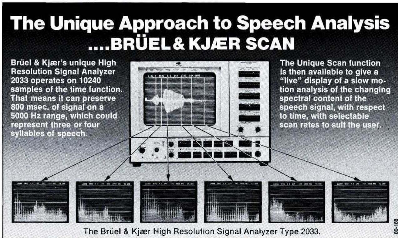
The Unique Scan function is then available to give a "live" display of a slow motion analysis of the changing spectral content of the speech signal, with respect to time, with selectable scan rates to suit the user.
