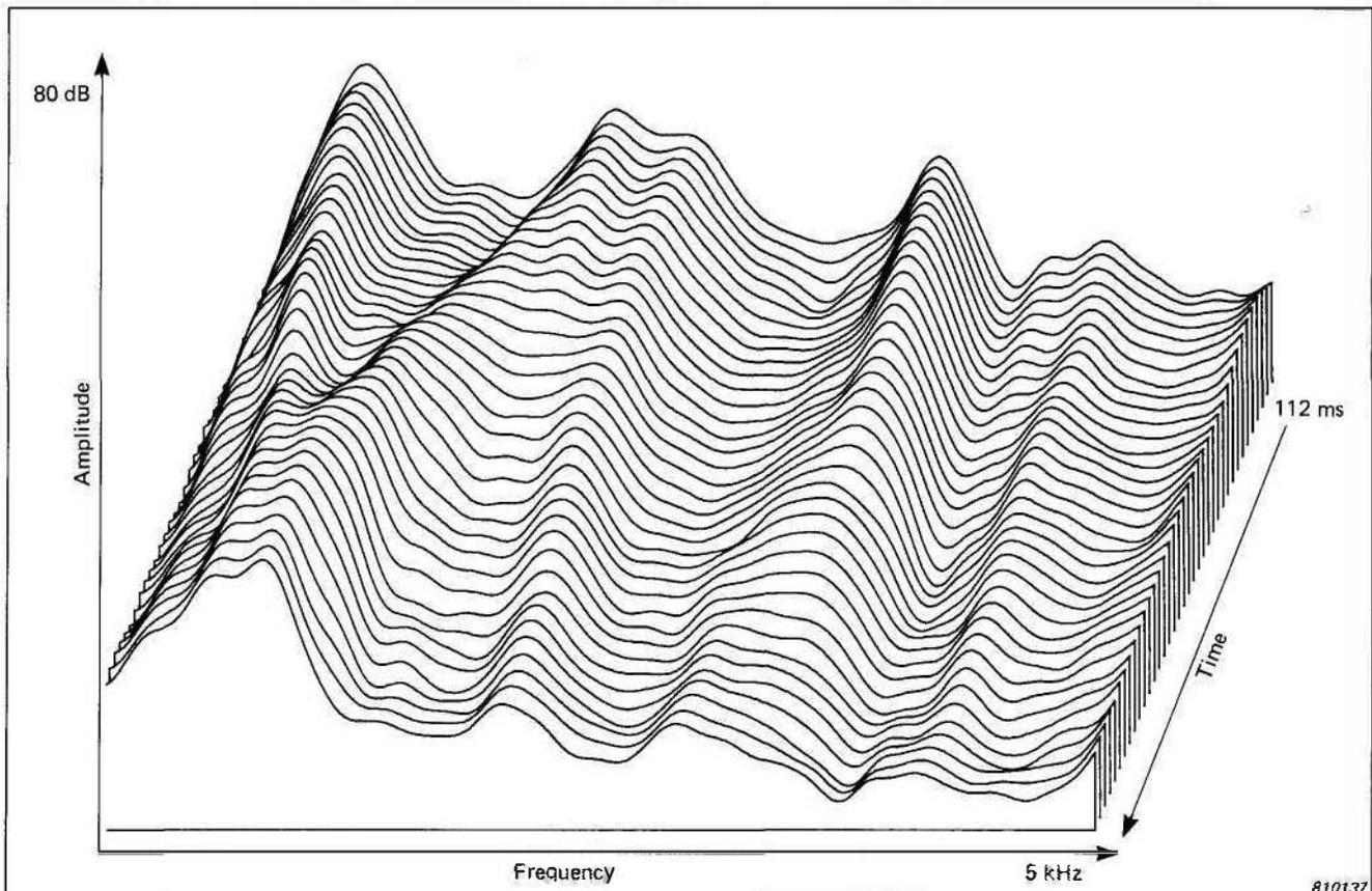
Fig.3. Short pass liftered scan spectrum of "ee" in "Montreal"
