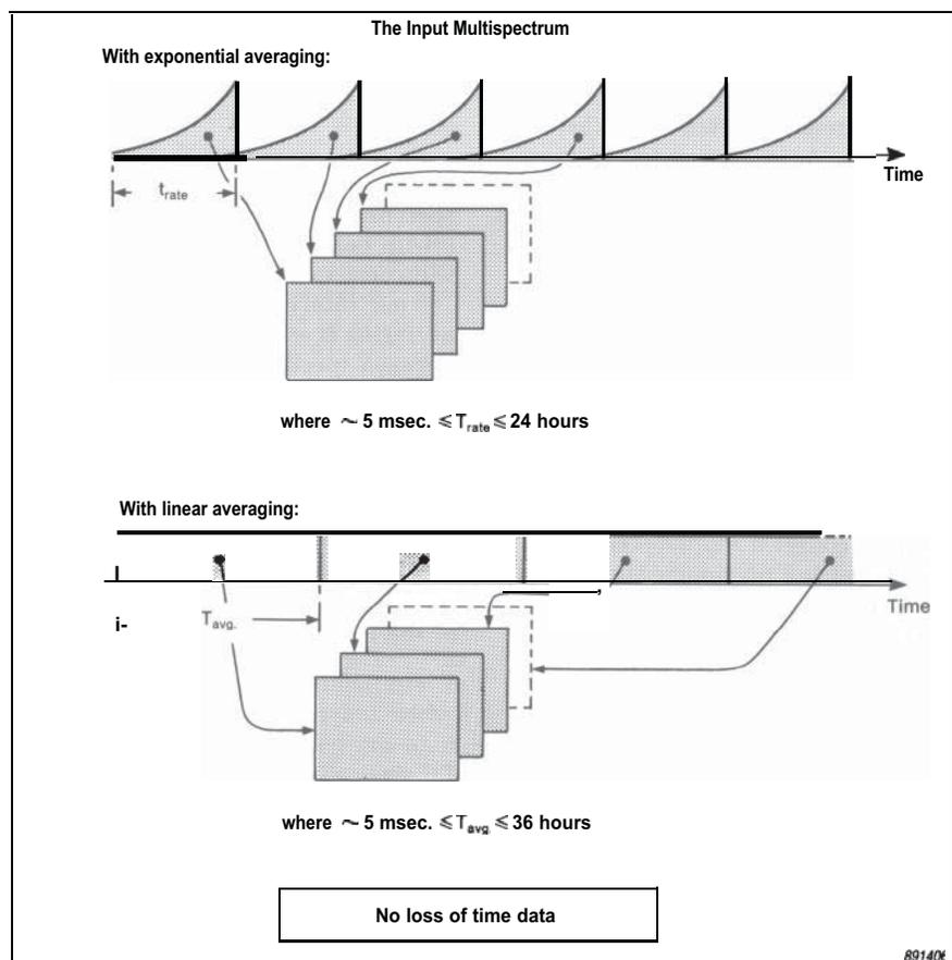
Fig. 1. Data collection in input multispectrum mode
