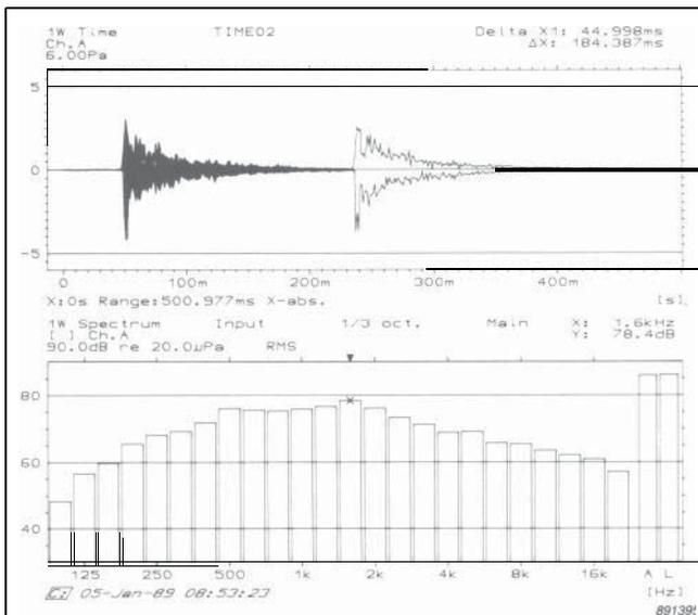
Fig. 15. An analysis of part of the time signal from Fig. 10. The part windowed out for analysis is highlighted using the delta cursor
