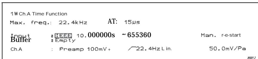
Fig. 20. Typical measurement set-up for time history mode
