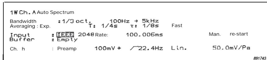
Fig. 10. Typical measurement set-up for spectrum history mode
