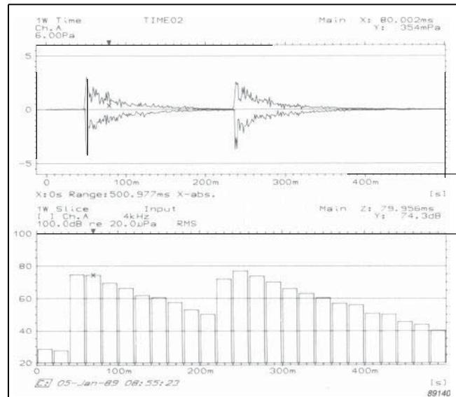
Fig. 16. An input multispectrum generated from the entire time signal captured in Fig. 10. A slice display of the 4 kHz 1/3 octave band is shown
