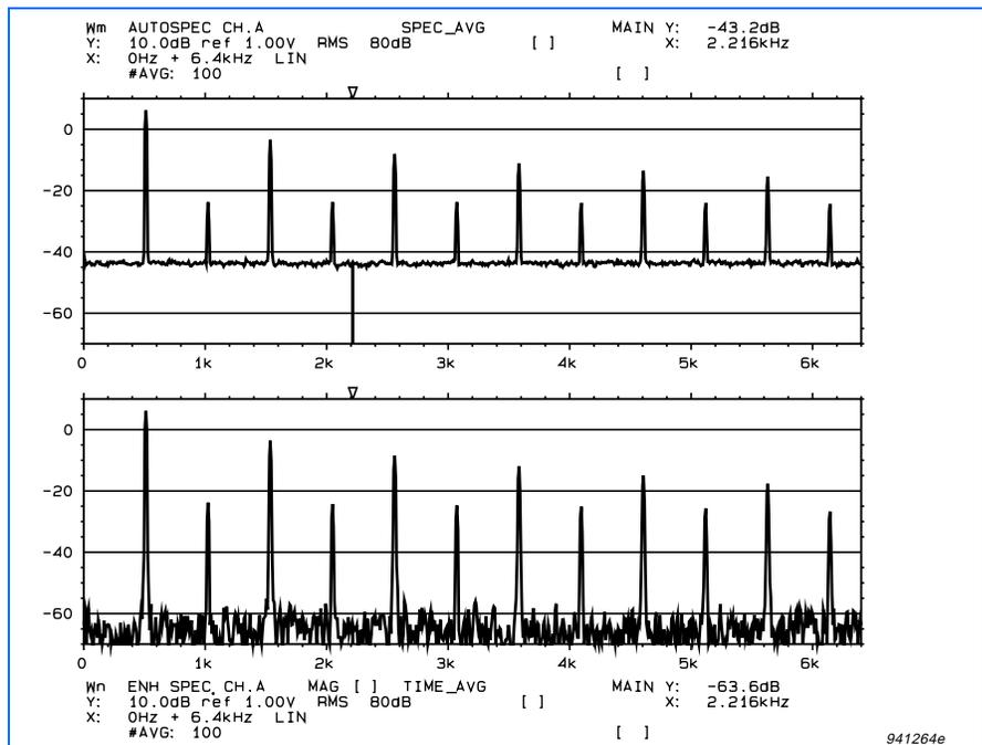
Fig. 3 Spectrum averaging (top) and signal enhancement (bottom)
