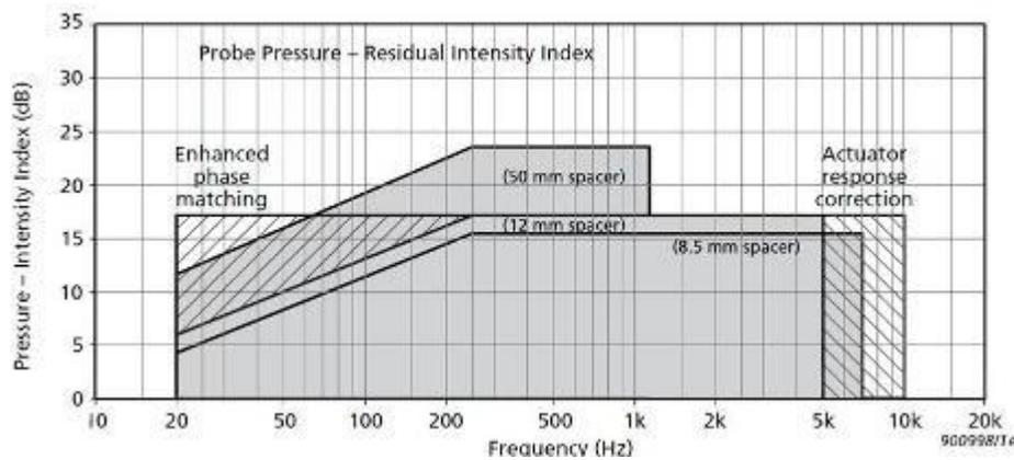
*Specified frequency and Pressure-Residual Intensity Index ranges for the probe (Pressure-Residual Intensity Index = Pressure level - Intensity level (measured in a closed coupler)). Frequency axis is in 1/3-octave centre frequencies.*
