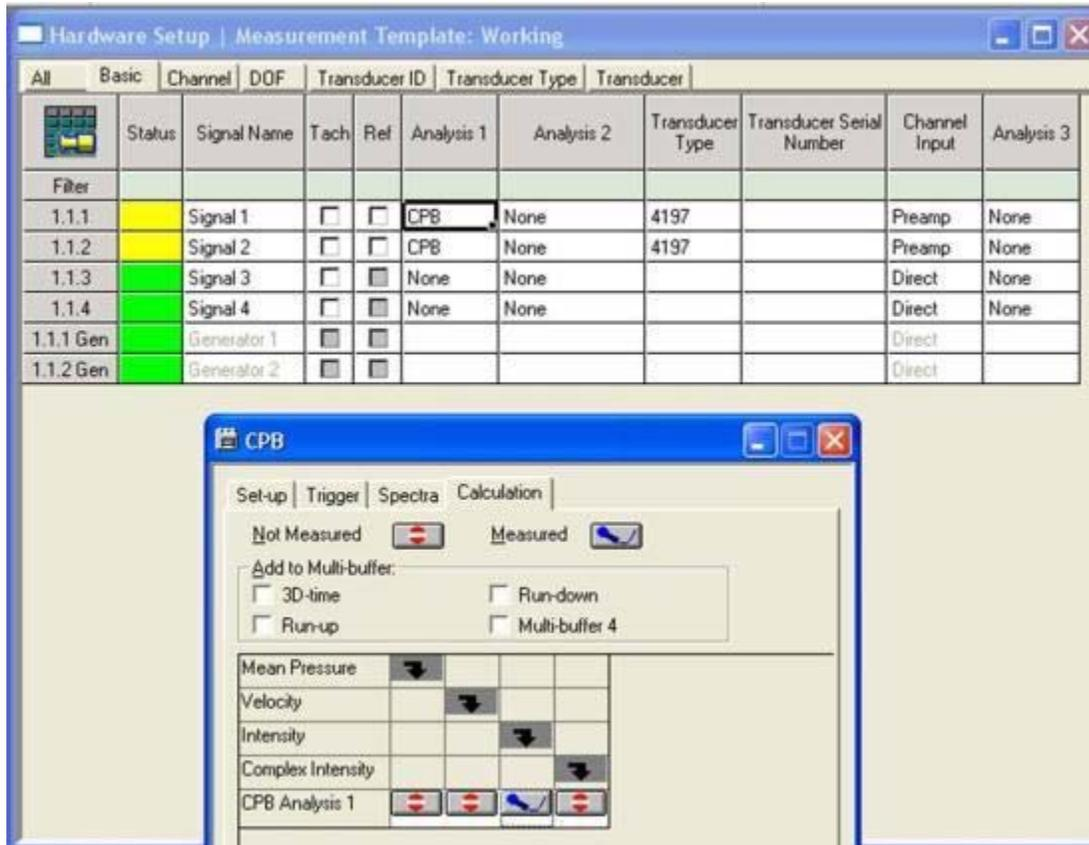
Please note that with the Transducer Type selected (here 4197), the Channels Input is automatically set to Preamp.
