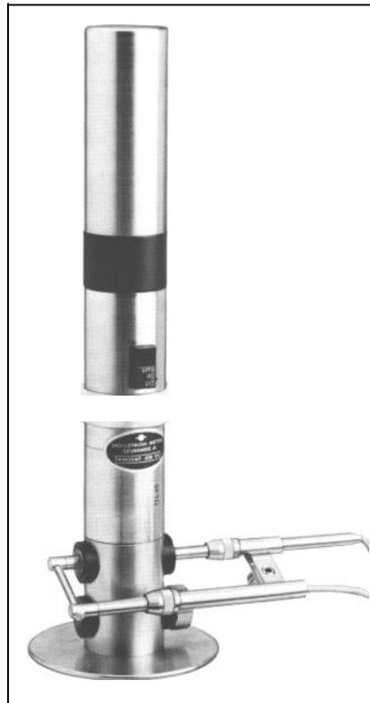
Fig. 4. Arrangement for pressure amplitude calibration
