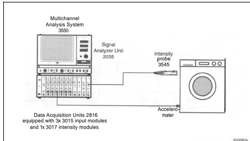
Fig. 4 Noise survey using the selective intensity technique
