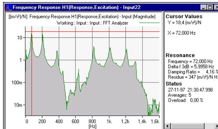
The resonance frequency is the easiest modal parameter to determine. A resonance is identified as a peak in the magnitude of the frequency response function, and the frequency at which it occurs is found using the analyzer's cursor as shown in Fig. 3.
