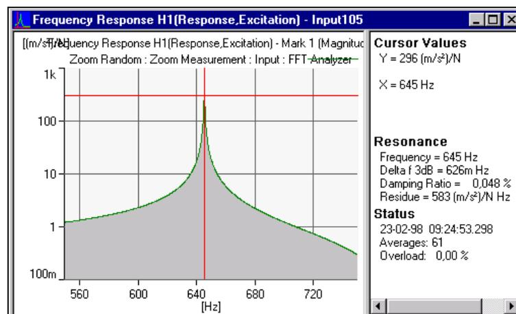
The frequency resolution of the analysis determines the accuracy of the frequency measurement. Greater accuracy can be attained by reducing the frequency range of the baseband measurement, for resonances at low frequencies, or making a zoom measurement around the frequency of interest, as shown in Fig. 4.
