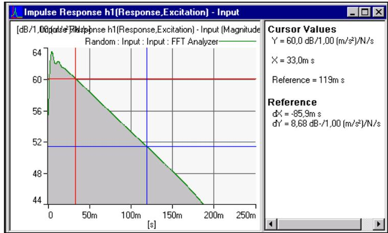
Since a simple structure behaves as a Single-Degree-of-Freedom system at each resonance, the impulse response function of the windowed resonance will show characteristic exponential decay  $\tau$ . By displaying the magnitude on a logarithmic scale the impulse response is represented by a straight line (see Fig. 6).
