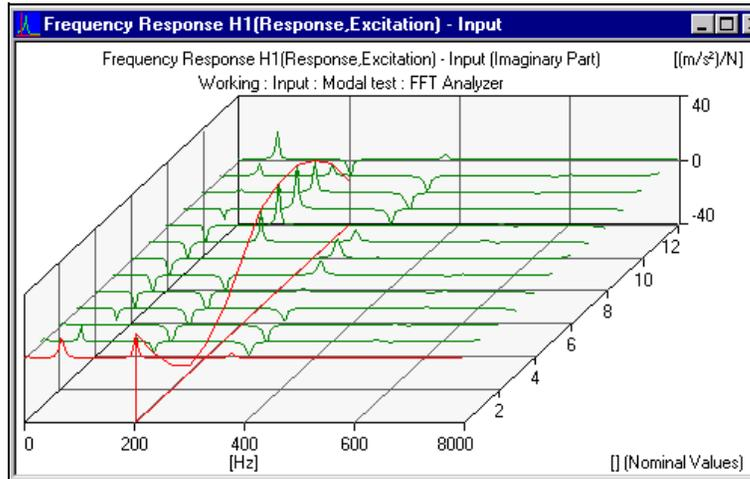
The mode shapes can be drawn by hand, or even simpler, the frequency response functions can be stored in a multi-buffer PULSE System and the mode shapes subsequently displayed by making slices in the multi-buffer as shown in Fig.8. This technique is only meaningful when the structure under test can be represented by DOFs on a straight line (i.e., a one dimensional structure).
