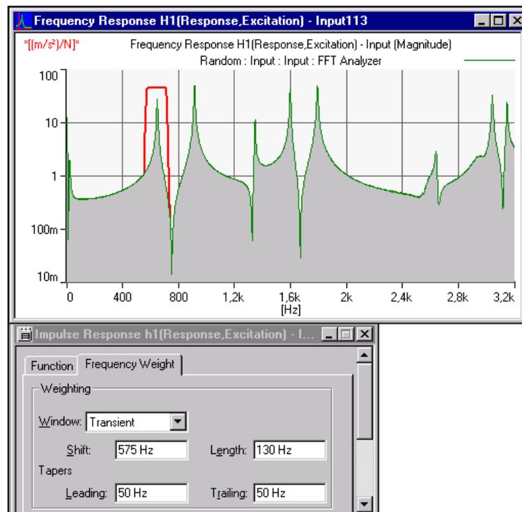
However, the PULSE System can be used to determine the damping ratio by an alternative method which requires no new measurements. By using a frequency weighting function (window) to isolate a single mode from the frequency response function (see Fig. 5), the impulse response function for that mode alone is easily produced. The magnitude (envelope) of the impulse response function can then be displayed by virtue of the Hilbert transform facility incorporated in the analyzers.
