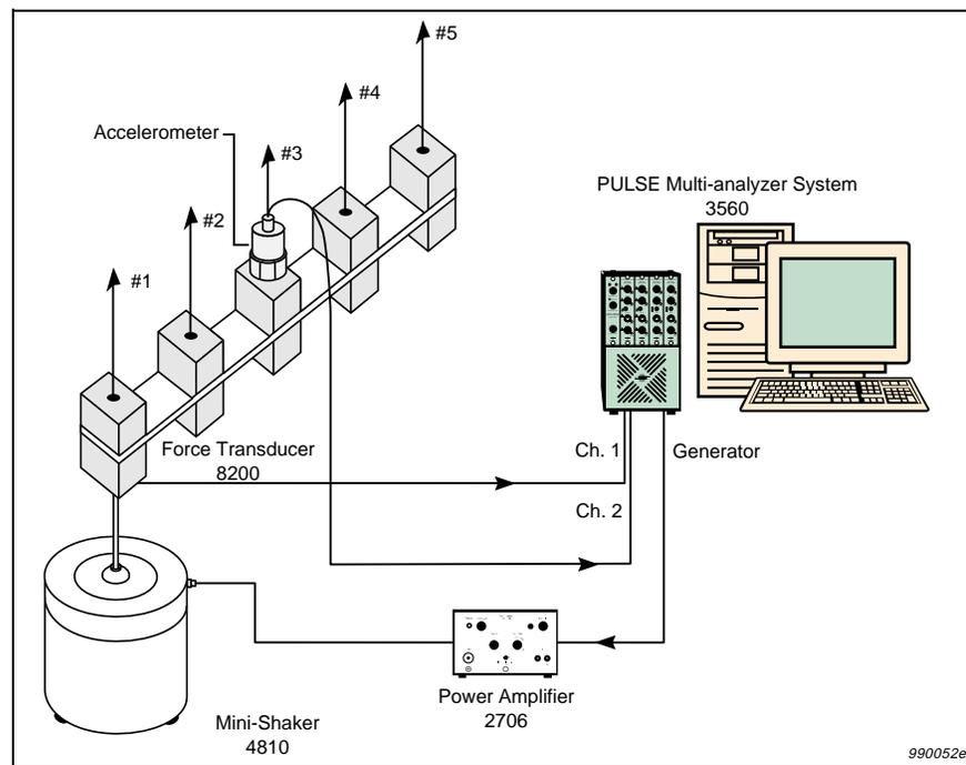
For structures defined with a large number of DOFs, the Multi-analyzer System Type 3560 can be equipped with up to eight four-channel modules (without expanding the physical dimensions of the system) to allow for easier and faster mobility measurements. Simultaneous measurement of up to 31 response signals and one force input signal can be performed, thereby greatly reducing the time needed to move the response accelerometer.
