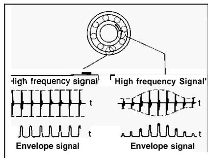
Fig 2. The modulation effect caused by a fault on the stationary and on the rotating race.
