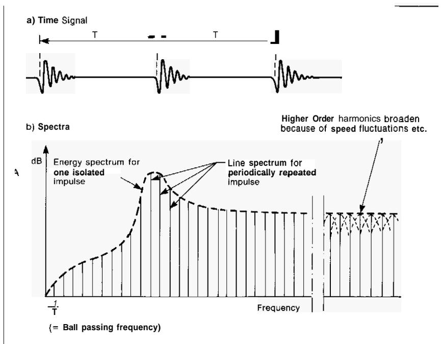
Fig. 1. Frequency spectrum for an idealized impact fault.
