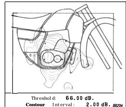
Fig. 7. Pressure contour plot. 1600 Hz twelfth octave band
