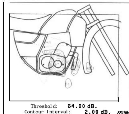
Fig. 6. Reactive intensity plot. 1600 Hz twelfth octave band
