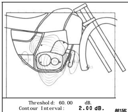
Fig. 5. Active intensity contour plot. 1600 Hz twelfth octave band
