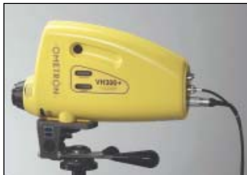
Fig. 11 Type 8329 – used to provide a reference signal
