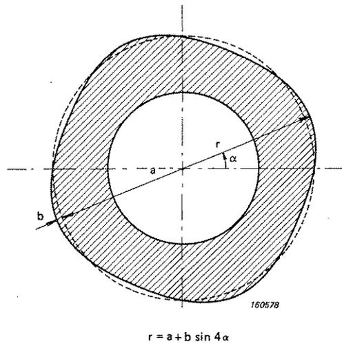
Fig.3.1. Cross-section showing the principle of operation
