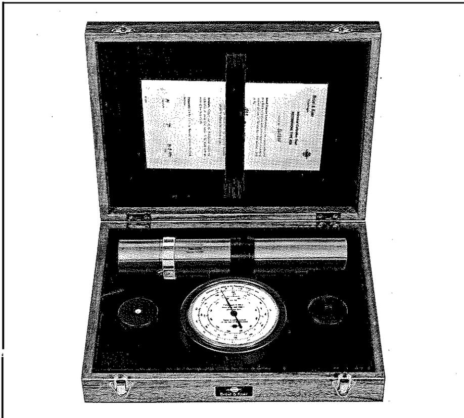
The Pistonphone is a compact battery-operated precision sound source, designed to enable quick and accurate overall calibration of sound measuring equipments. It produces a sound pressure level of 124 dB at a frequency of 250 Hz.
