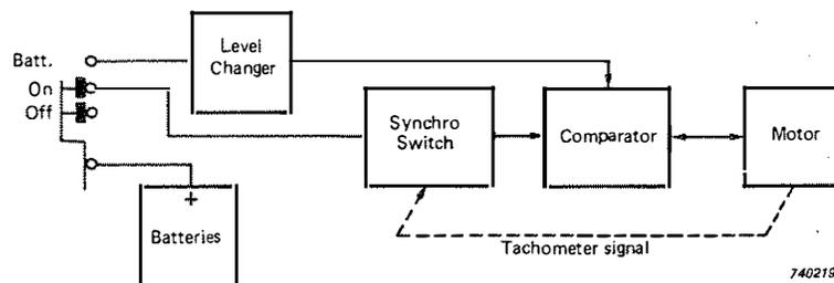
**Fig. 3.6.** *Block diagram of motor control system*
