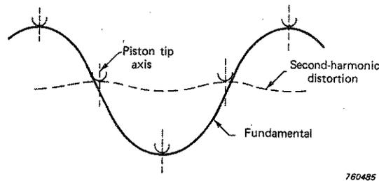
Fig.3.3. Second-harmonic distortion when cam shape follows Eqn. 3.1
