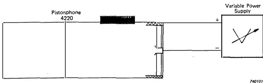
Fig. 2.4. Connection of an external variable power supply
