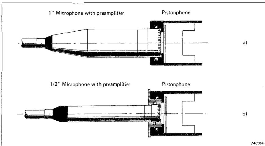
Fig.2. Mounting B & K microphones on the Pistonphone
