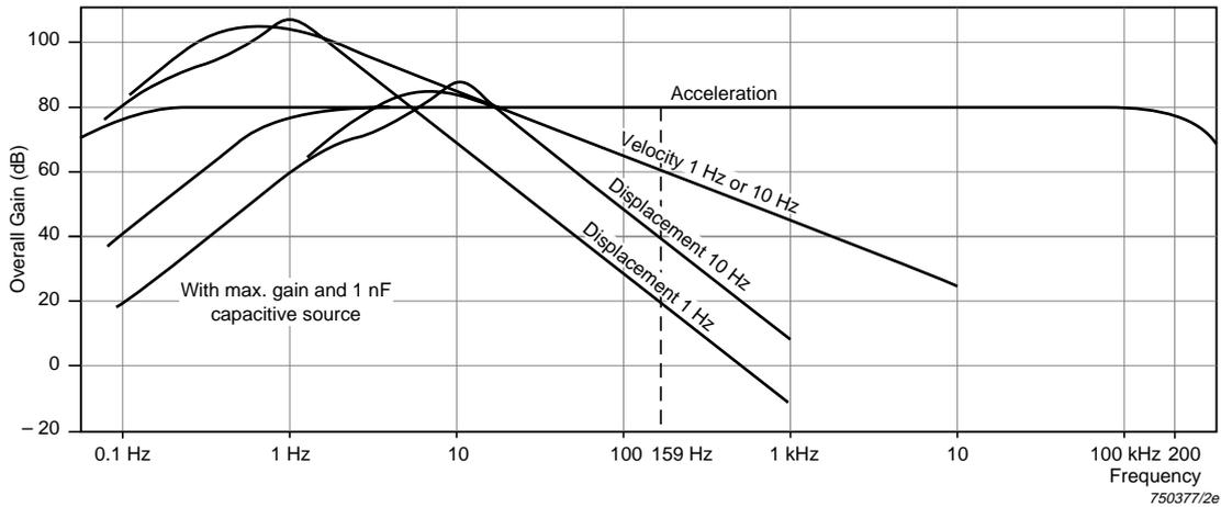
Fig 3 Frequency response curves in linear position (acceleration), and with integrators for velocity and displacement. Low-pass filters at 100 Hz, 1 kHz, 3 kHz, 10 kHz and 30 kHz are not shown
