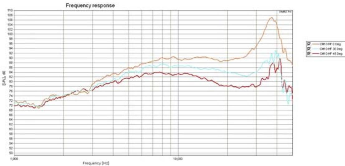
**Figure 2b – Response of CM10 tweeter without crossover at 0°, 30° & 45° horizontally off axis**
