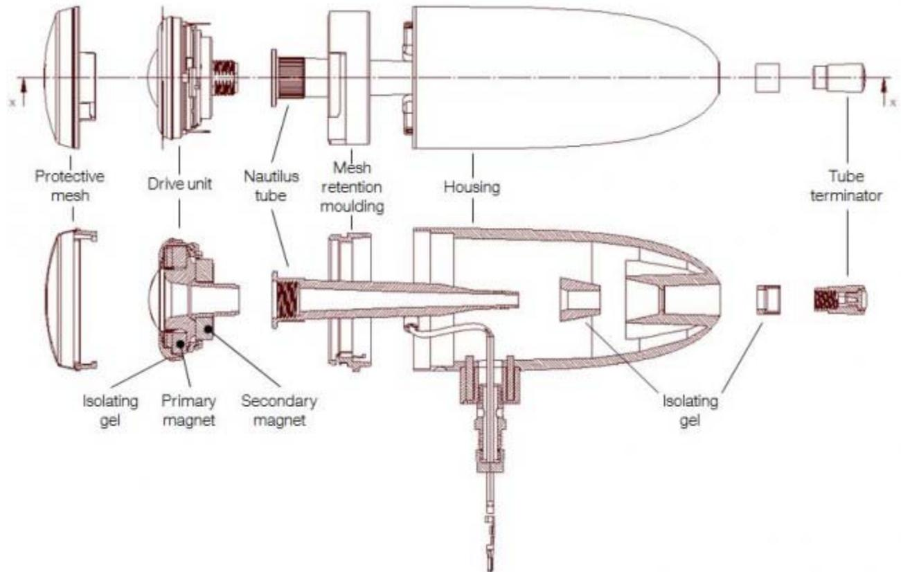
Figure 3 – Exploded illustration of CM10 tweeter construction
