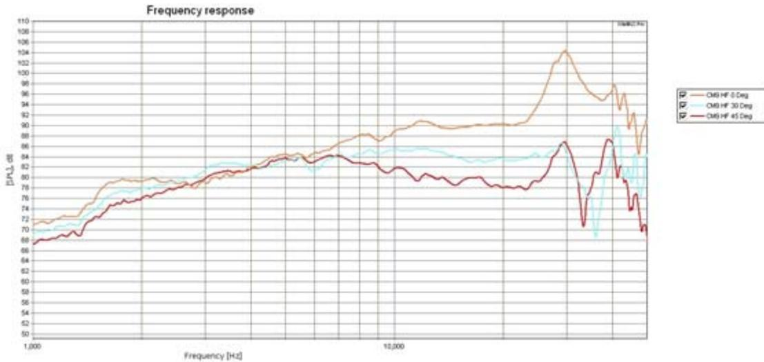
**Figure 2a – Response of CM9 tweeter without crossover at 0°, 30° & 45° horizontally off axis**
