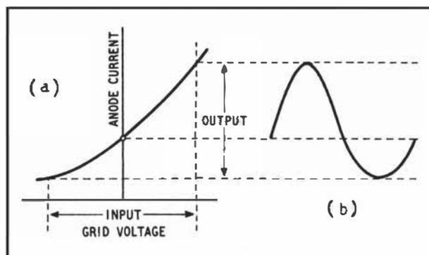
Fig. 2. Typical valve characteristic (a) with the curvature somewhat exaggerated we hope, showing the resulting distortion of a sine wave (b).
