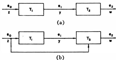
Fig. 1—(a) Usual configuration for correcting nonlinear distortion by complementary distortion.  $z$ ,  $y$ , and  $w$  are normalized signal variables. (b) A multiply connected configuration for correcting nonlinear distortion generated in the left-hand circuit.
