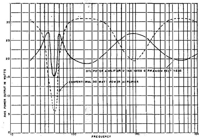
FIG. 7. Power output in watts versus frequency for a. the output-transformerless amplifier, when a 1N158 germanium rectifier is used (solid curve); b. a conventional 30-watt power amplifier (dashed curve).
