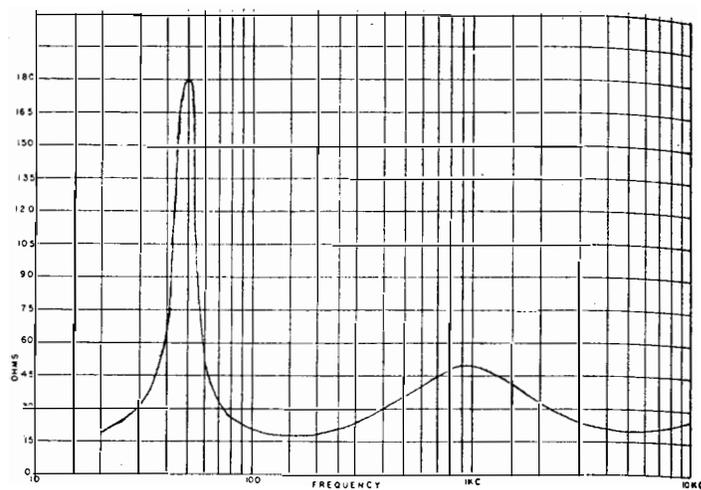
FIG. 5. Measured impedance curve of the author's LC-1A loudspeaker in 10-cu-ft infinite baffle.
