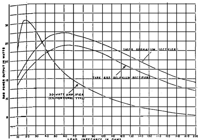
FIG. 6. Power output of output-transformerless amplifier at the overload point, plotted as a function of load impedance (when germanium and selenium rectifiers are used). Curve A represents the power output of a conventional 30-watt amplifier; curve B, the power output of the OTL amplifier with a 6S2 selenium rectifier; curve C, the output of the OTL amplifier when a 1N158 germanium is used.
