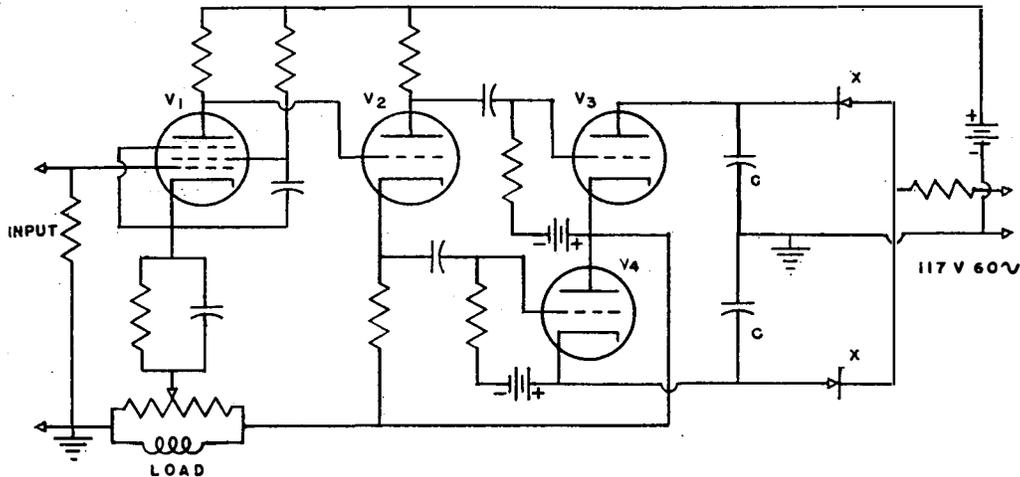
FIG. 1. Basic schematic of the output-transformerless power amplifier.
