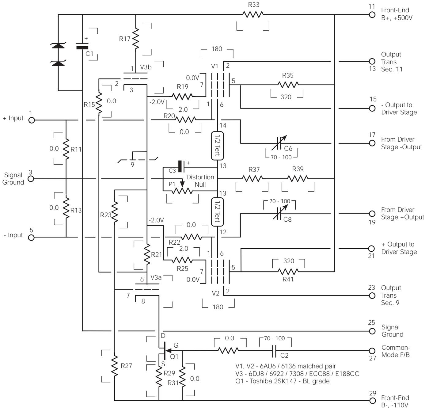
The suppressor grids are connected to the secondary of the output transformer for the reasons outlined on page 6 of *Audio Note* 23.1, under the section heading "The Output Stage".
