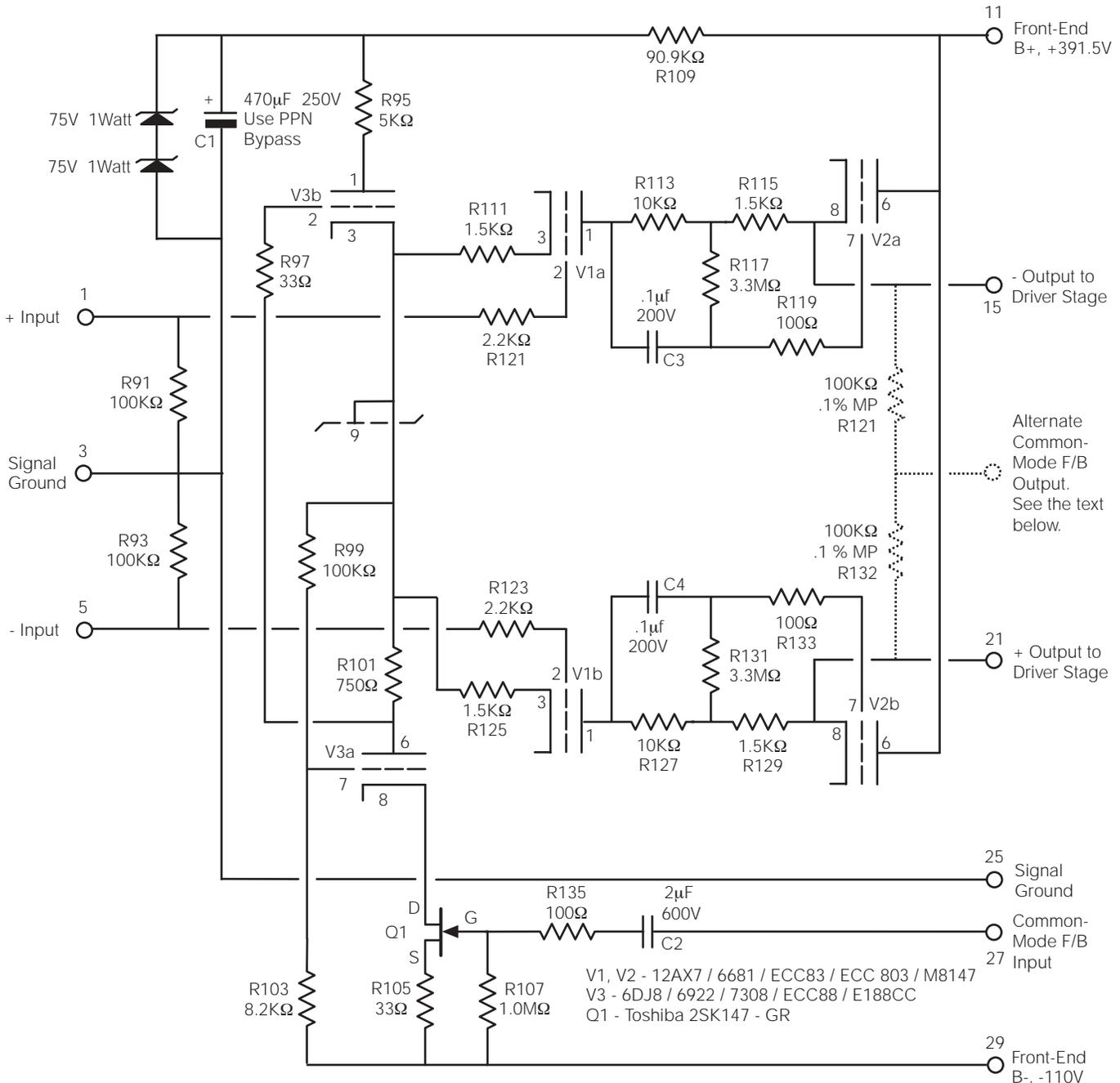
**Figs. 6 & 7** The alternate "no loop feedback" version of the SC 280.1 front-end is shown in these two figures. As with the "loop feedback" version, the differential amplifier shown above uses an active current-source to create an accurately push-pull pair of signals to drive the output stage. These are created from an input signal that can be either single-ended or balanced.
