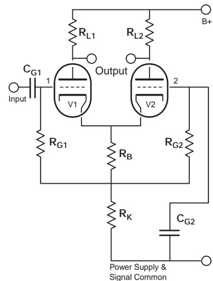
Fig. 6. One method of eliminating the negative voltage supply for the cathode return.  $R_B$  is tapped off the total cathode resistance at the desired bias point.
