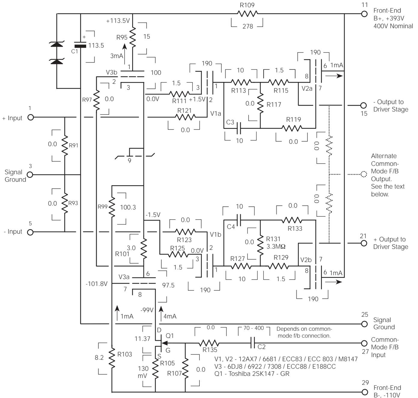
Disconnect the "Common-mode F/B Input" from the 100K $\Omega$  matched-resistor pair in the driver stage and connect it to the "Alternate Common-mode F/B Output" shown in dashed lines in the front-end schematic. Don't use driver stage outputs 17 and 19.
