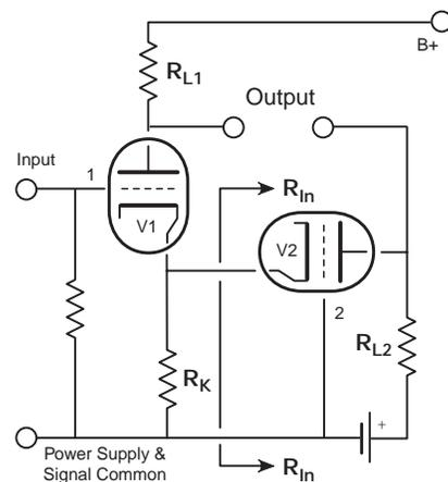
Fig. 3. The “long-tailed-pair” redrawn to show the grounded-grid operation of V2.
