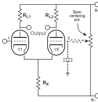
Fig. 5. When using the "long-tailed-pair" to feed the balanced deflecting plates of a cathode-ray oscilloscope, the grid of V2 may be returned to an adjustable, DC divider to restore the beam to the center of the 'scope screen.
