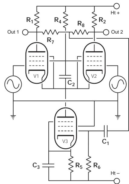
Fig. 4. A differential amplifier-stage with additional feedback.
