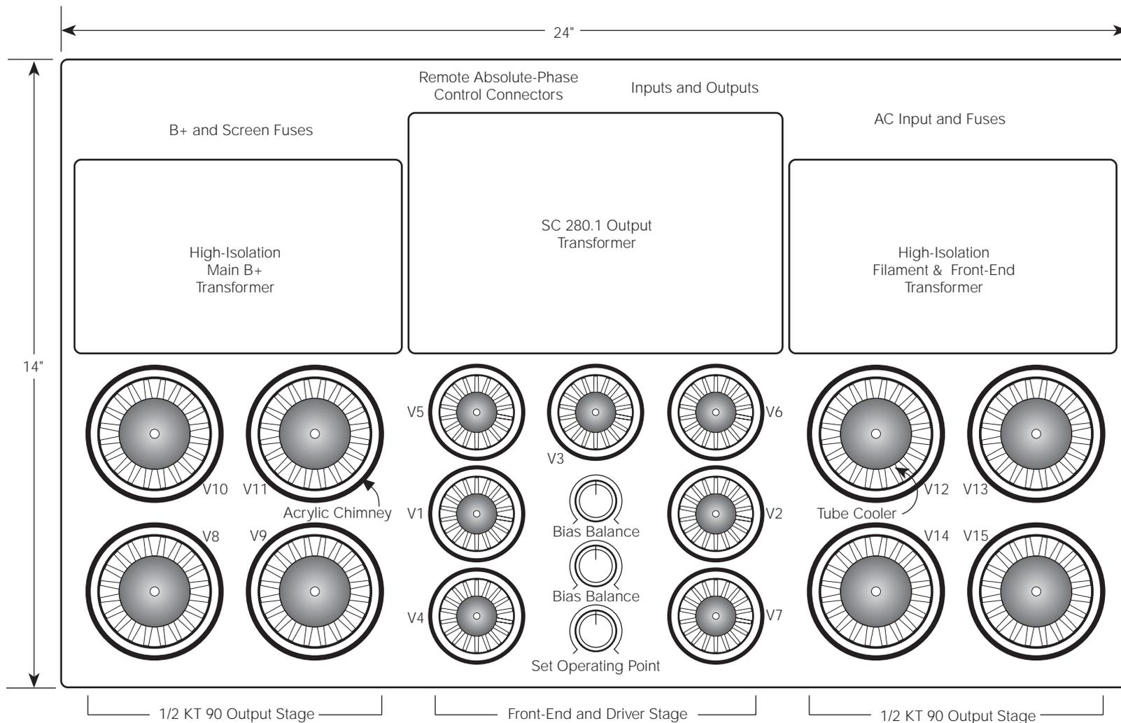
Fig. 1 - Mechanical Layout - Plan View
