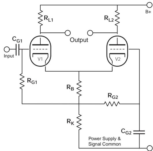
Fig. 7. One method of eliminating the negative-voltage supply for the cathode return.  $R_B$  is tapped off the total cathode resistance ( $R_B + R_K$ ) at the desired bias point.
