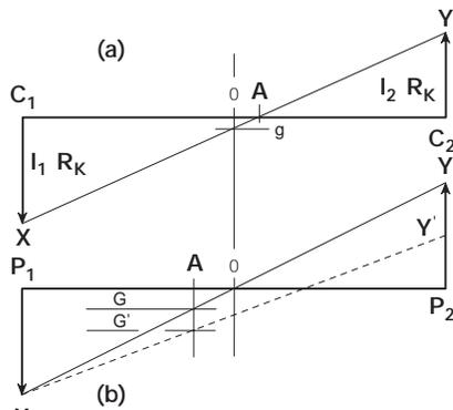
Fig. 2. (a) Current-see-saw diagram of the “long-tailed-pair”. (b) See-saw diagram of balanced-voltage phase inverter reprinted from last month’s article for comparison with the balanced-current type.
