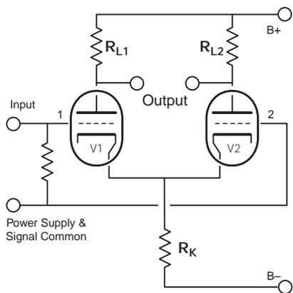
Fig. 1. Circuit of the “long-tailed-pair” cathode-coupled phase inverter.
