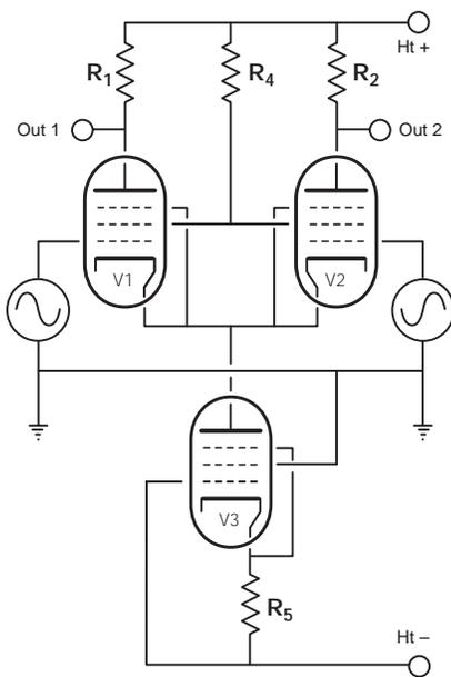
Fig. 2. A conventional differential amplifier-stage using pentodes.
