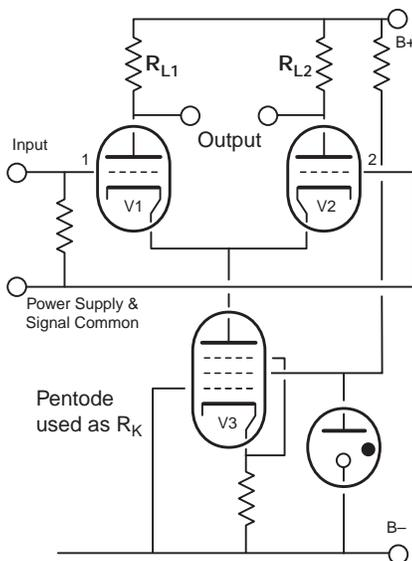
Fig. 4. A high-impedance pentode as a common-cathode-resistor swamps out variations in tubes 1 and 2 that might unbalance the phase-inverter currents.
