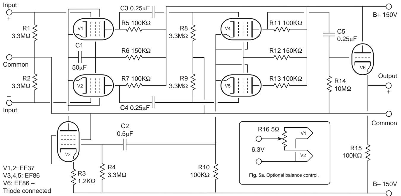
Fig. 5. A practical differential amplifier-stage.
