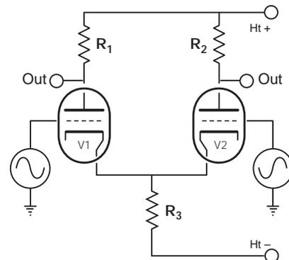
Fig. 1. A simple differential amplifier-stage.
