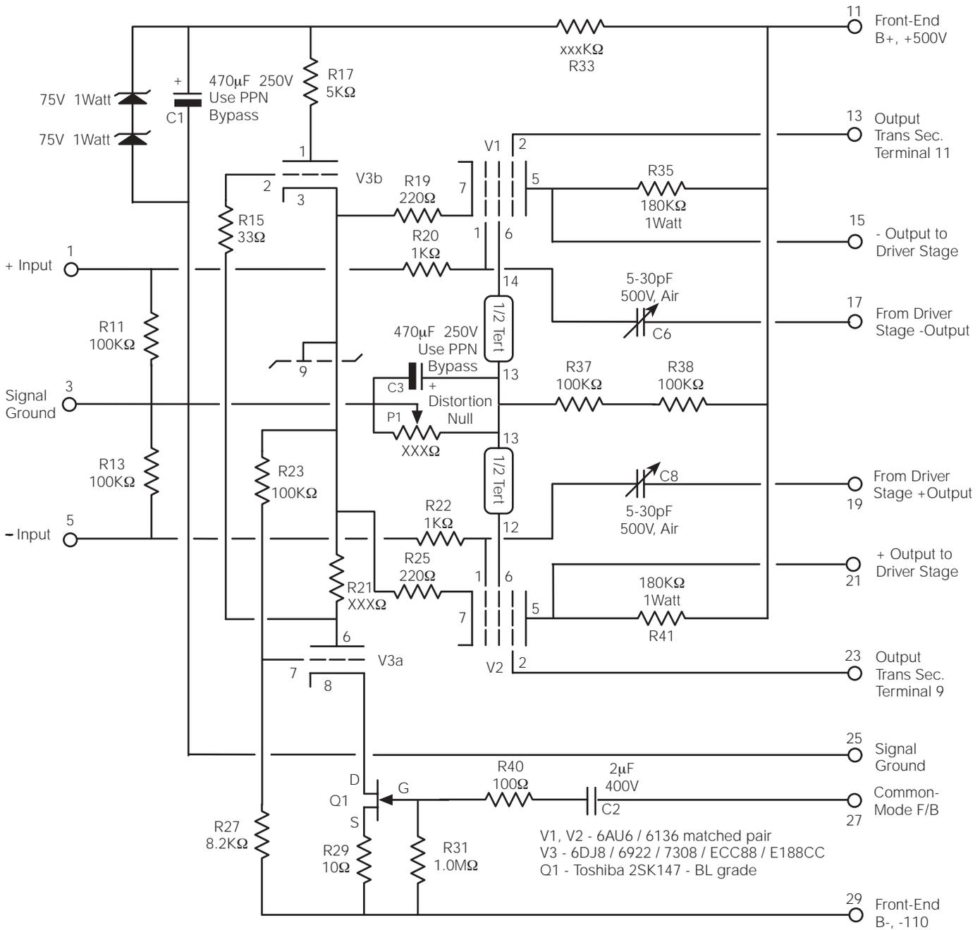
**Figs. 4 & 5.** The front-end of the "loop-feedback version" of the SC 280.1 is shown in these two figures.
