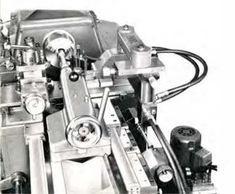
The wide range of attachments available for use on this lathe includes thread chasing, taper turning, spherical turning, grinding and hydraulic profiling equipment (illustrated). Spindle speed reduction units and various types of toolbox are also available.
