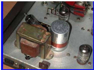
Using the smallest bit possible, drill a hole for each new lead wire next to each terminal it will attach to. Push the leads through the phenolic disk, seating the new electrolytics on the disk. Wrap the leads around their terminals, and route the ground to the can, adding a bit of spaghetti tubing if needed. Solder the new leadouts to the terminals.
