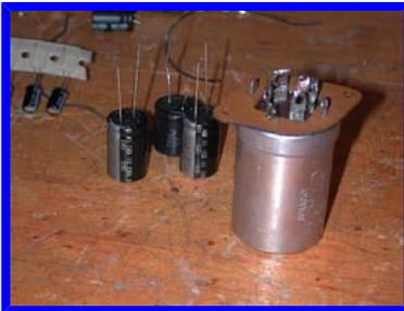
First, gather the new electrolytics you will use to replace the existing guts of the can. They must fit inside the can, so arrange them as they will be placed in the can and make sure they don't exceed the height or diameter of the can, plus some wiggle room. Note the advice on cap selection in the previous section.
