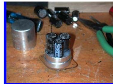
I prefer to add some RTV around the capacitors to stabilize them in the can. Now you must seal up the can you cut open. I've completed quite a few of these rebuilds by just taping the can together with copper tape, but lately I've added a thin
