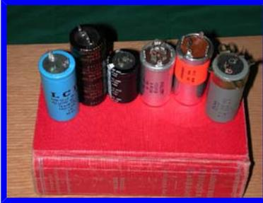
From left to right, we have a LCR computer capacitor, an Elna Cerafine computer type (unfortunately no longer in production), a Panasonic TSHA snap-mount capacitor, a new-production Aero-M twistlock, a NOS Mallory twistlock, and a good-but-used Elna removed from equipment.
