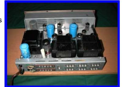
Mounting these caps requires a clamp screwed to the chassis, and you'll usually have to add some holes for the clamp attachment, and perhaps enlarge the clearance hole for the connection lugs. Clamps can be found at [Mouser Electronics](#) for about 50c. Typically, there are fewer sections compared to the original twistlocks, so some of the sections must be moved into the chassis.
