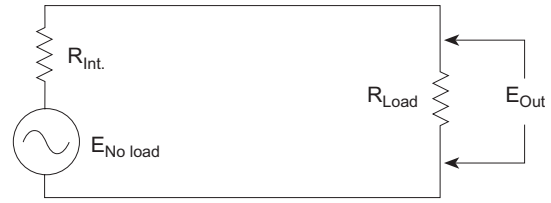
Fig. 1. Equivalent output circuit.
