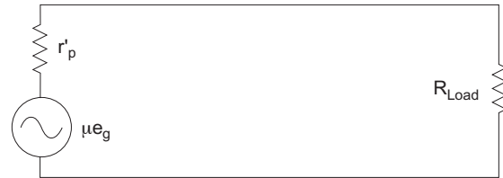
Fig. 2. Schematic of the equivalent plate circuit of the output stage.
