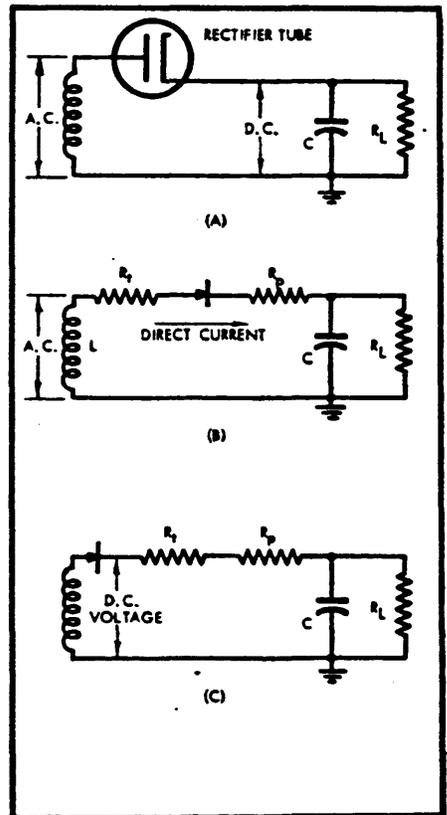
Fig. 6. (A) Power supply schematic. (B) Equivalent of (A), with transformer replaced by  $L$  and  $R_t$ , tube replaced by unidirectional element and plate resistance,  $R_p$ . (C) Positions of  $R_t$  and rectifier reversed, a permissible operation in a series circuit. When  $R_t$  is connected, direct current flow causes voltage drop in  $R_t$  and  $R_p$ .
