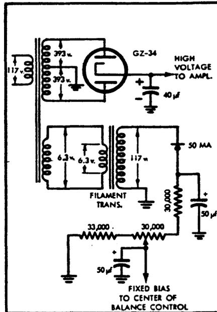
Fig. 5. Fixed bias supply using standard components.
