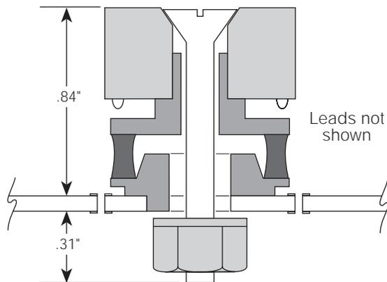
**Fig. 3.** The standard profile, PC mounting, vertical ISO-SOCKET is shown above. The contacts are silver plated brass, the socket body is white ceramic and Sorbothane is used for the decoupling elastomer.
