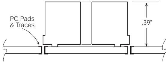
**Fig. 1.** The seated height of a standard, PC mounted 7/9-pin tube socket is shown above. Use this to gauge the increase in the seated height of tubes fitted into any of the ISO-SOCKETS shown on this page.
