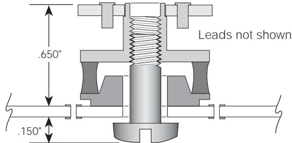
**Fig. 2.** The low profile, PC mounting, vertical ISO-SOCKET is shown above. The contacts are gold plated brass, the socket body is blue G10 fiberglass and Sorbothane is used for the decoupling elastomer.
