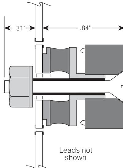
**Fig. 5.** The standard profile, PC mounting, horizontal ISO-SOCKET is shown above. The contacts are silver plated brass, the socket body is white ceramic and silicone foam is used for the decoupling elastomer.
