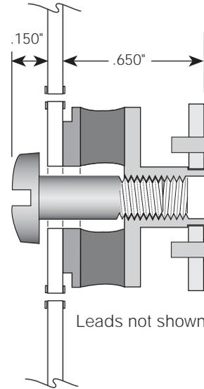
**Fig. 4.** The low profile, PC mounting, horizontal ISO-SOCKET is shown above. The contacts are gold plated brass, the socket body is blue G10 fiberglass and silicone foam is used for the decoupling elastomer.
